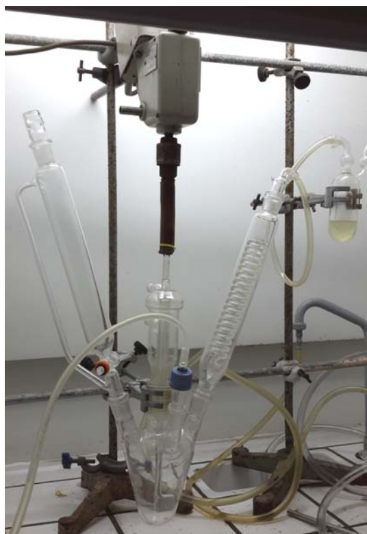
Figure SM 13.8.1 – Reaction set-up apparatus for tetraethylammonium bis(1,3-dithiole-2-thione-4,5-dithiol) zincate
