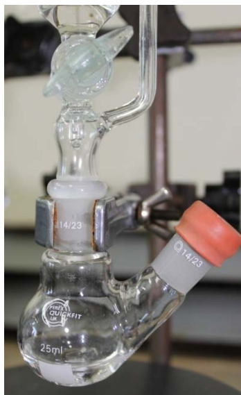
Figure SM 13.7.5 – Slow dropwise addition of an acetophenone solution using a dropping funnel
