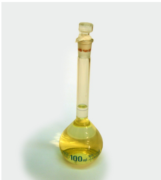
Figure SM 13.4.1 – Diethyl ether solution of \text{MoO}_2\text{Cl}_2(\text{H}_2\text{O})_2 .
