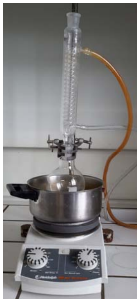
Figure SM 13.8.3 – Reflux set-up apparatus
