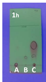
Figure SM 13.4.6 – TLC using n -hexane as eluent (A: diphenyl sulfoxide, B: triphenylphosphine, C: reaction mixture) at 1 hour of reaction.
