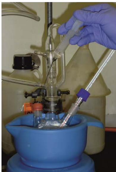
Figure SM 13.5.16: Setup in Dewar, addition of reagent
