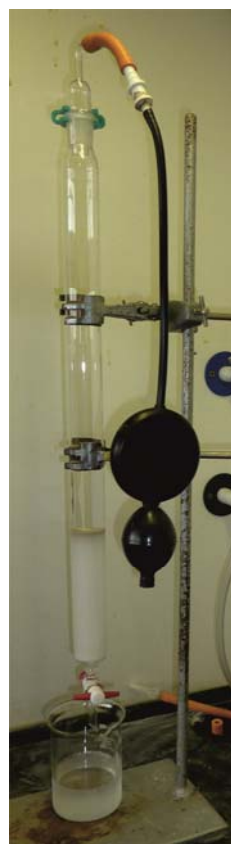
Figure SM 13.5.18: Packed column with bellows
