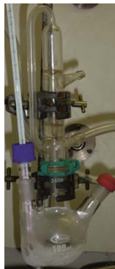
Figure SM 13.5.17: Setup after removal of cooling bath
