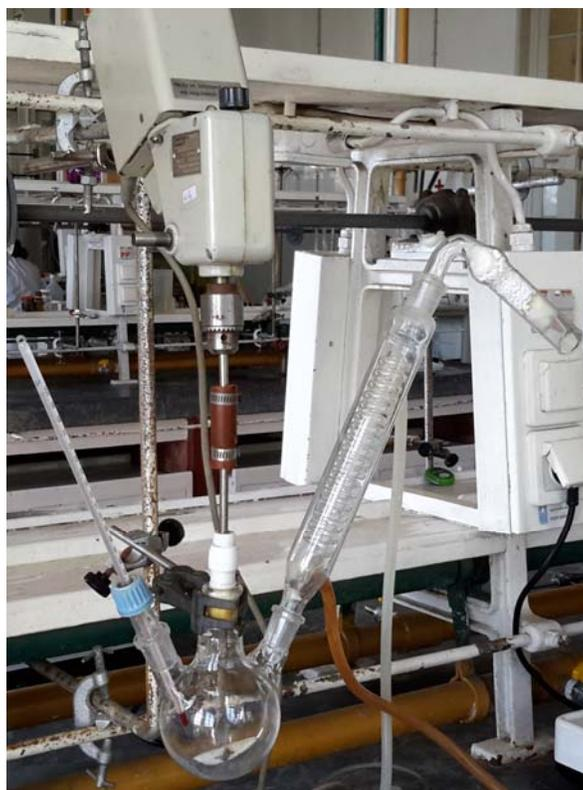
**Figure SM 4.1.2.2.2** – Reaction set-up apparatus for *o*-hydroxydibenzoylmethane
