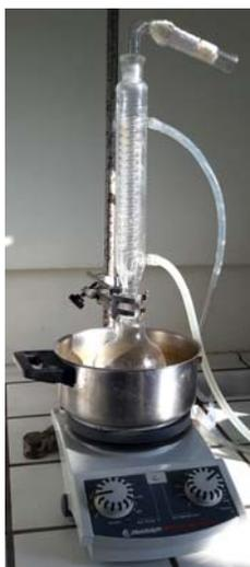
**Figure SM 4.1.2.2.1** – Reaction set-up apparatus for o-benzoyloxyacetophenone
