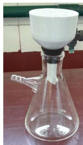
**Figure SM 4.1.2.2.3** – Copper funnel (previously heated by flame) for hot filtration during flavone recrystallization from petroleum ether and vacuum filtration set-up
