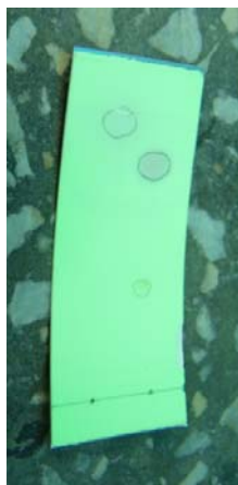
Figure 5.1.6.1. TLC plate of naphthalene and the student's 1-nitronaphthalene in UV lamp 254nm
