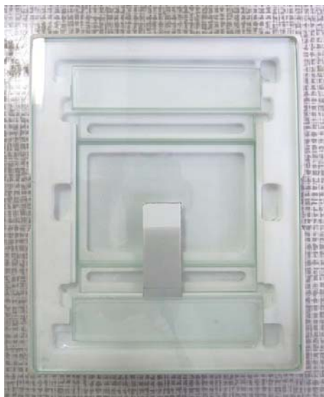
Figure 5.1.6.2. Vertical chamber used for TLC of 1-nitronaphthalene
