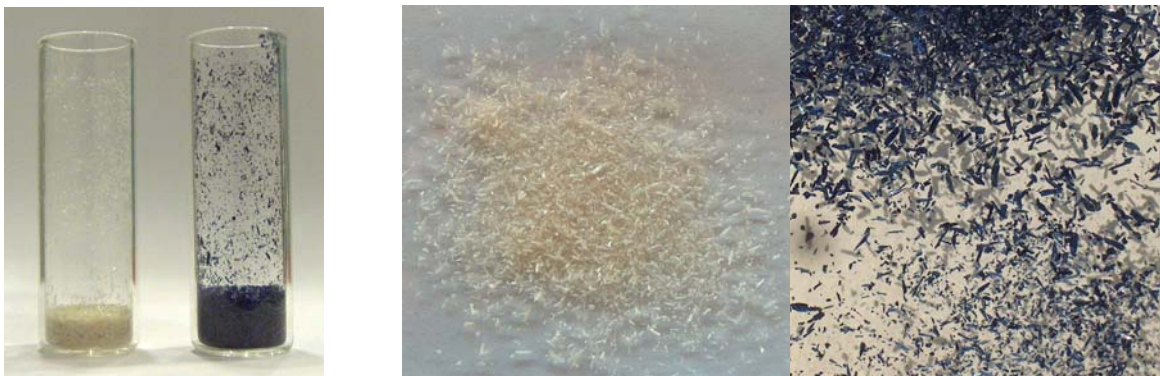
SM 5.1.3.1 - Crystals of 2-(2,4-dinitrobenzyl)pyridine stored at dark (sandy) and after sun light exposition (dark blue)
