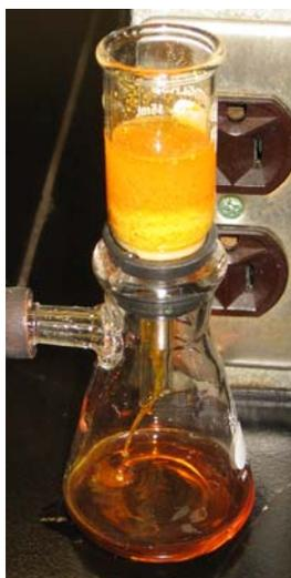
**Figure SM 7.1.1.** Formation of the diazonium tosylate (left) and washing of the crude 1-iodo-2-nitrobenzene with sodium sulfite solution (right).
