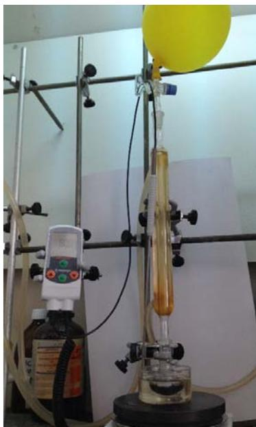
**Figure SM 7.9.3** - Synthesis of 3-styryl coumarin (step3). Water condenser into the round-bottomed flask under a nitrogen atmosphere.
