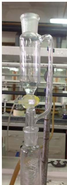
**Figure SM 8.1.2** – Setup after removal of heating bath and addition of ethyl iodide.
