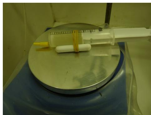
**B.** Artisanal orbital shaker with a stir bar attached around the syringe.
