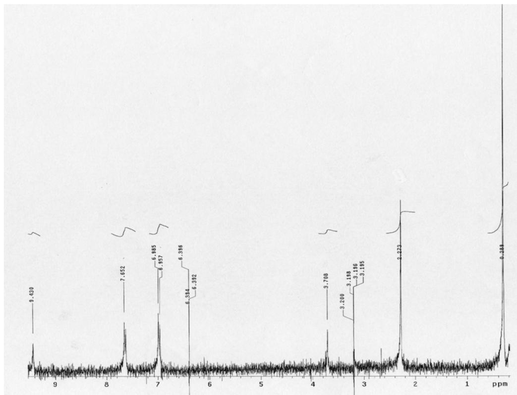
**Figure SM 8.1.6** - <sup>1</sup>H NMR of *p*-hydroxyacetanilide (300 MHz, CDCl<sub>3</sub>/DMSO-d<sub>6</sub>)
