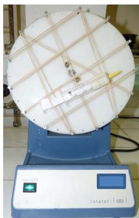
**A.** Orbital shaker with a vertical rotating tray.
