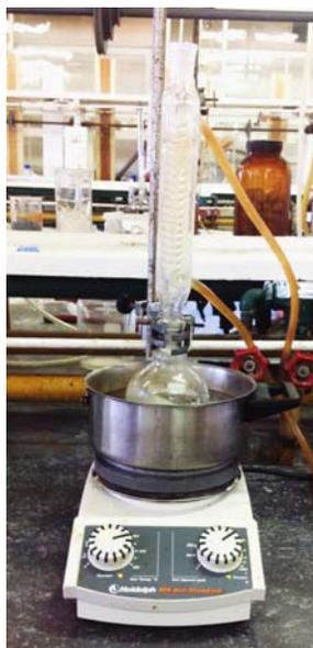
**Figure SM 8.1.1** – Reflux setup.
