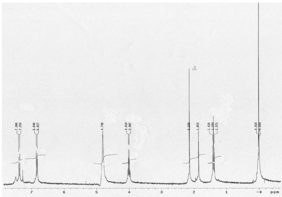
**Figure SM 8.1.8** -  $^1\text{H}$  NMR of dulcin (300 MHz,  $\text{CDCl}_3$ )
