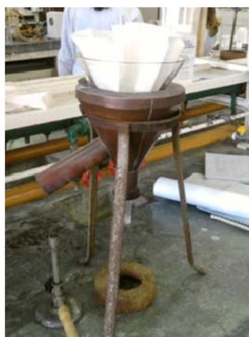
**Figure SM 8.1.3** – Dulcin recrystallization from water. Heating plate and copper funnel (previously heated by flame) for hot filtration
