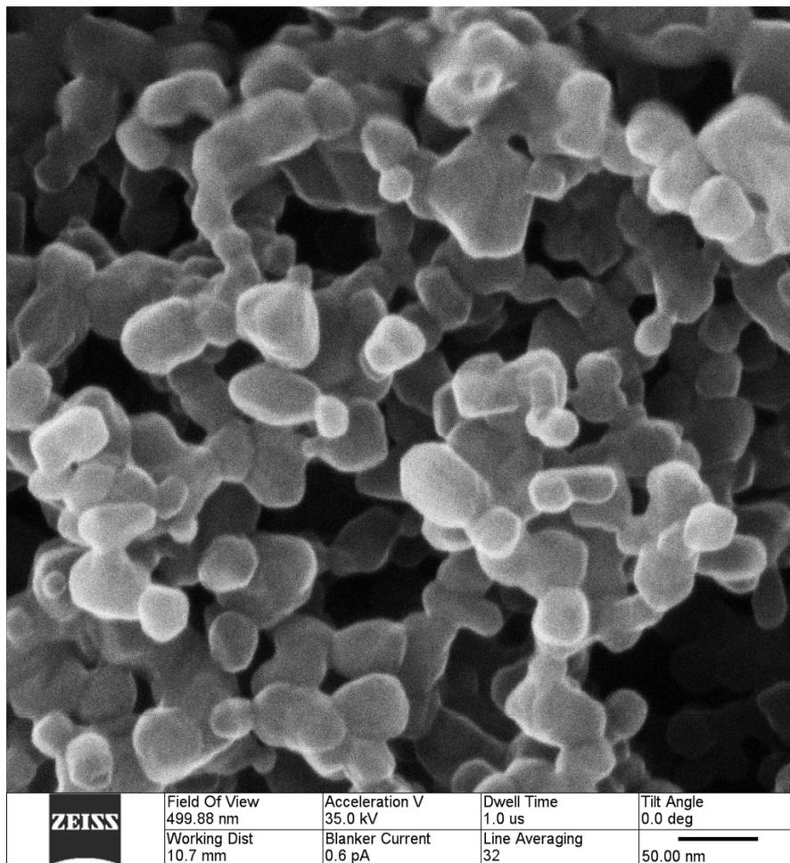
**Fig. ESI 2** HIM images of  $\text{CuCo}_2\text{O}_4$  films on stainless steel mesh used for catalytic test.
