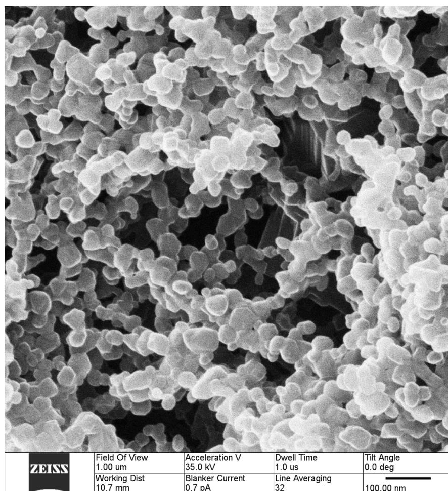
**Fig. ESI 1** HIM images of CuCo<sub>2</sub>O<sub>4</sub> films on stainless steel mesh used for catalytic test.
