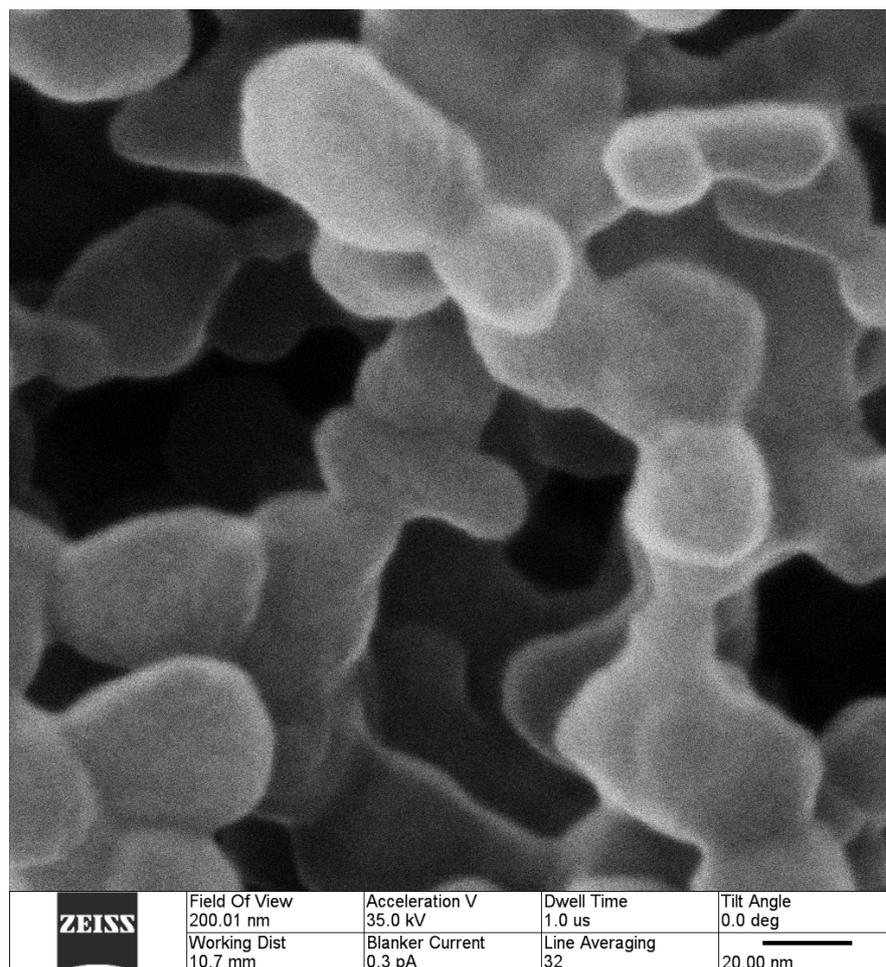
**Fig. ESI 3** HIM images of  $\text{CuCo}_2\text{O}_4$  films on stainless steel mesh used for catalytic test.
