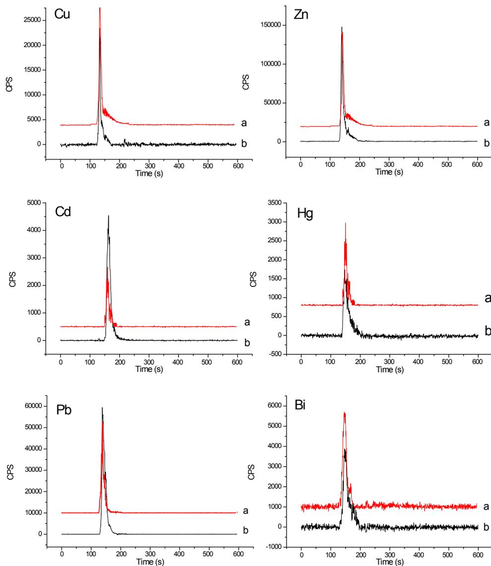
167 **Fig. S5** HPLC-ICP-MS chromatograms for the eluent from the chip-based MSPME of
