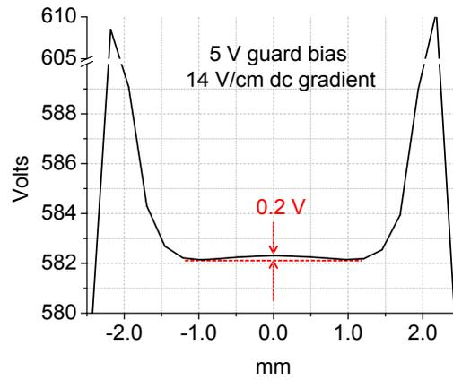
Figure S2: At 14 V/cm gradient and 5 V guard bias, the potential minima occurs at  $X = \pm 1.43$  mm from each board (or  $\sim 1.0$  mm from center axis between the boards). The inter-board gap is 4.85 mm.
