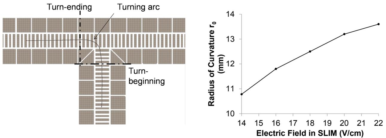
Figure S4. Left panel shows the averaged ion trajectory (excluding Brownian motion) in the SLIM tee at 10 V guard bias and 14 V/cm drift field, indicating the point of beginning and ending of the turn. Right panel shows the radius of curvature of the turning arc for different drift fields at 10 V guard bias. These radii values were used in the theoretical expression to evaluate the theoretical resolving power obtained during an ion turn at different drift fields.
