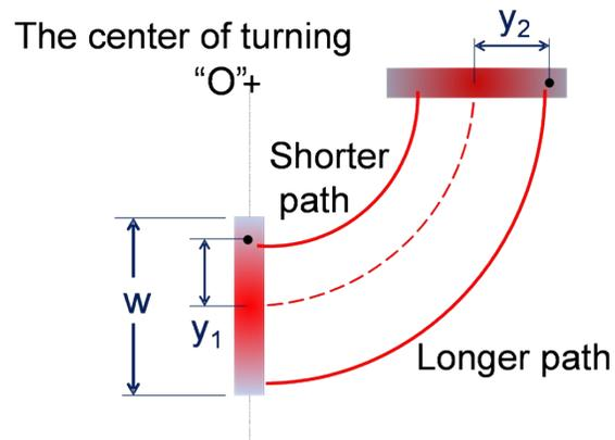
Figure S3: Ion beam (marked in gradient of red color) of width  $w$  turning through 90 degrees. The ions farther away from the turning center traverse a longer path and take longer time, whereas the ions closer to the turning center take a shorter time. This results in an increase in the standard deviation of the arrival time distribution of the peak after the turn, which is being referred to as the "race track" effect.
