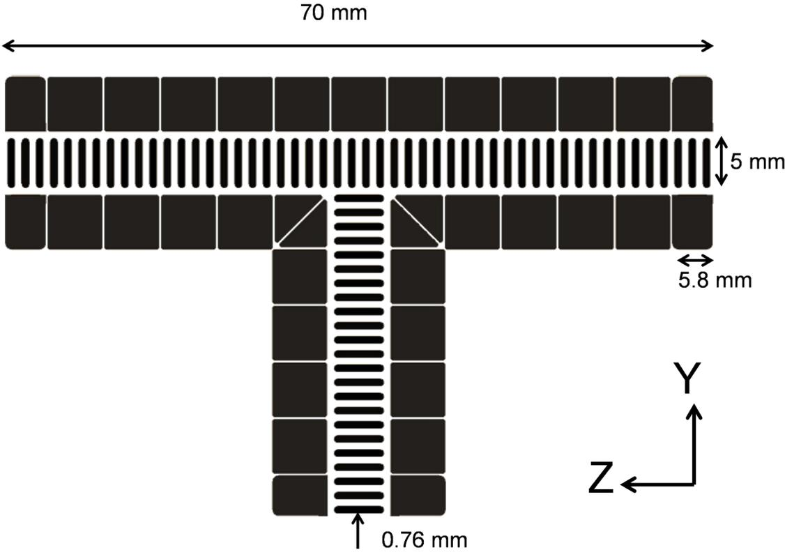
Figure S1: SLIM tee component electrode design. Two SLIM PCB-constructed boards are arranged parallel to each other, to form a single unit of tee. The straight tee units (discussed elsewhere[1, 2]) can be used in conjunction with tee to form flight paths of required dimensions.
