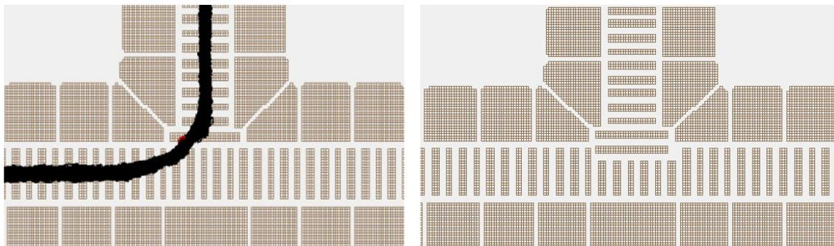
Figure S5: Left panel shows the elongated electrode design and right panel shows the elongated and insert electrode design
