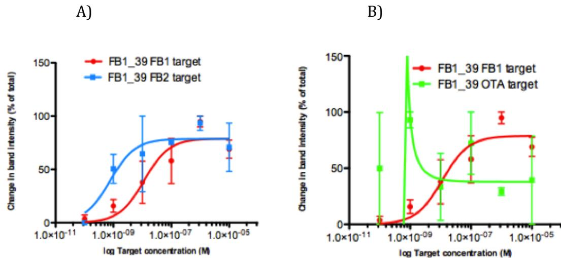
**Figure S7. A)** Binding isotherms generated from Band E of the DNase I digestion assay showing the  $K_d$  of  $FB_1$  39 with  $FB_1$  and  $FB_2$ , and **B)** Binding isotherms generated from Band E of the DNase I digestion assay showing the  $K_d$  of  $FB_1$  39 with  $FB_1$  and OTA. Binding isotherms were generated using GraphPad Prism non-linear regression one-site specific binding.  $K_d$  of binding to  $FB_2$  was  $0.77 \pm 0.65$  nM; no binding observed to OTA.
