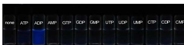
Figure S4. Fluorescence colour (under a 365 \text{ nm} light) changes of ZnL ( 5 \mu\text{M} ) in 10 \text{ mM} aqueous HEPES buffer solution ( \text{pH} = 7.2 ) with 50 \mu\text{M} of different anions (from left to right: none, ATP, ADP, AMP, GTP, GDP, GMP, UTP, UDP, UMP, CTP, CDP, CMP).
