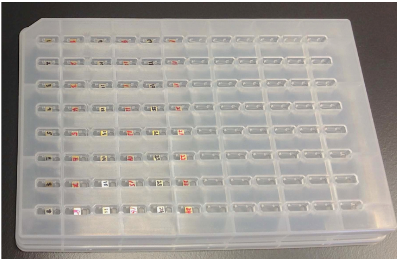
Fig. S5 Custom-made 96-well plate for incubating microchips carrying tissue sections in solutions of library compounds. Each chip set (AD and normal brain) is placed side by side and is treated with the same solution.
