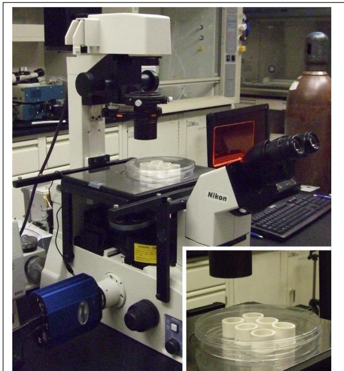
*Supplementary figure 2: Overall imaging set-up for the observation of wrinkle patterns generated by cancerous cells. Inset shows 6 devices which each contain ultra-thin membranes, culture media and cells.*
