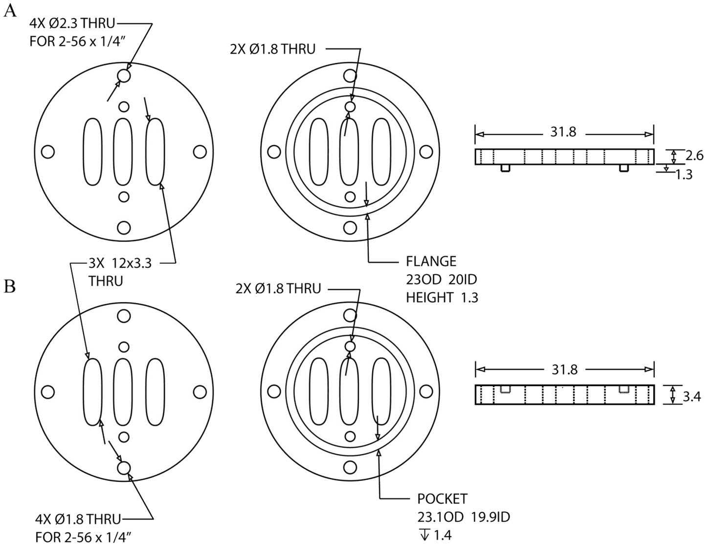
**Figure S3.** Detailed schematic showing each side of the A) top and B) bottom halves of the stainless steel holder used in the paper-based chemotaxis assay. Each holder contained three  $12 \times 3.3$  mm channels, four (2.3 mm) holes for combining both halves with four ( $2-56 \times 1/4$  in.) screws, and two (1.8 mm) holes for alignment purposes during assay assembly. All values are in units of millimeters unless otherwise indicated.
