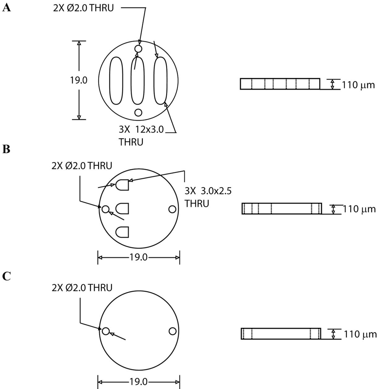
**Figure S2.** Schematic of cellulose acetate transparency films, designed in Adobe Illustrator: A) open design, B) partially open design (oxygen gradient), and C) closed design. The 2 mm holes on each side of the scaffold are present for assembling purposes. All values are in units of millimeters.
