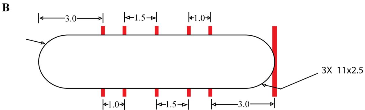
**Figure S1.** Schematic of a paper-based scaffold, designed in Adobe Illustrator: A) entire scaffold, and B) a single channel from the scaffold. The 2 mm holes on each side of the scaffold are present for assembling purposes and the red lines, which are wax printed, guide seeding and image alignment. All values are in units of millimeters.
