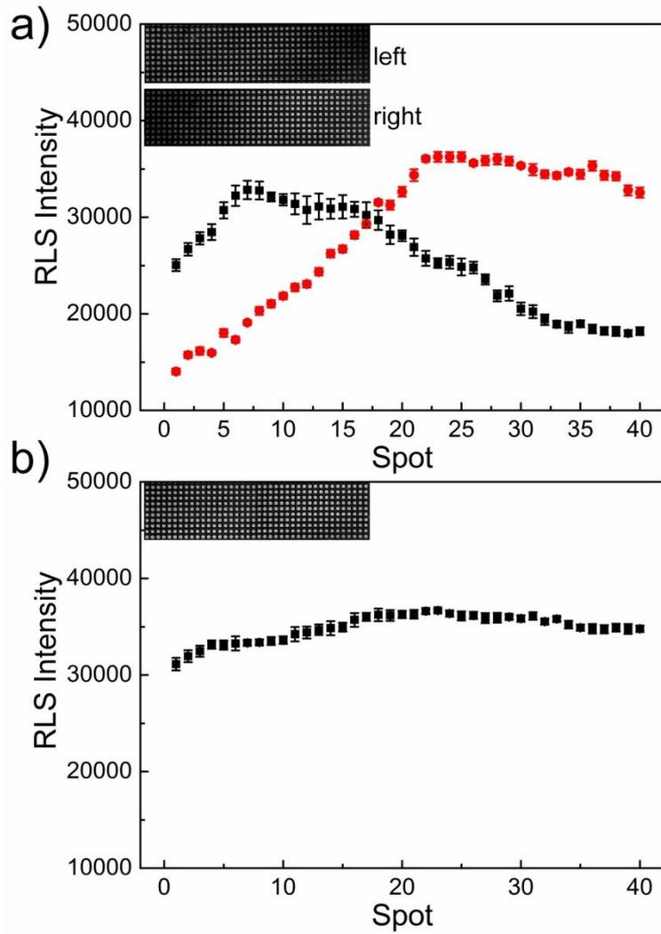
**Fig. S4.** RLS images and corresponding RLS intensities of 40×10 spots on the DNA microarray detected by PW-RLS scanner with (a) light incident from left (■) /right (●) side of the microarray slide and (b) light incident from both sides of the microarray slide.
