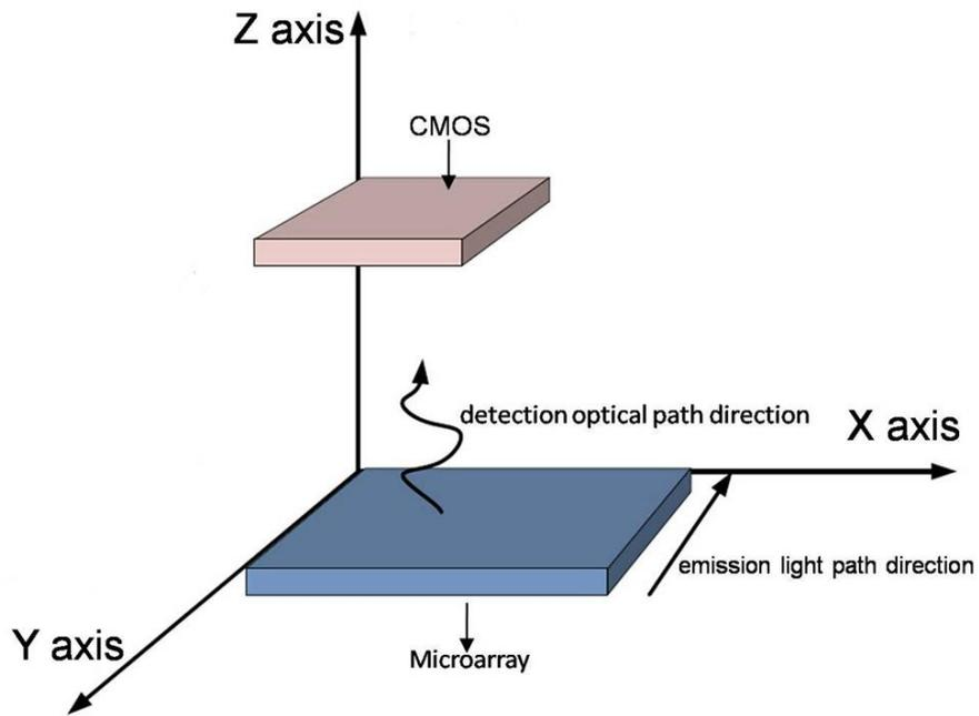
**Fig. S3.** The directions of the detection of optical path and the emission light path. The detection of optical path is perpendicular to the microarray and the emission light path is parallel to the microarray.
