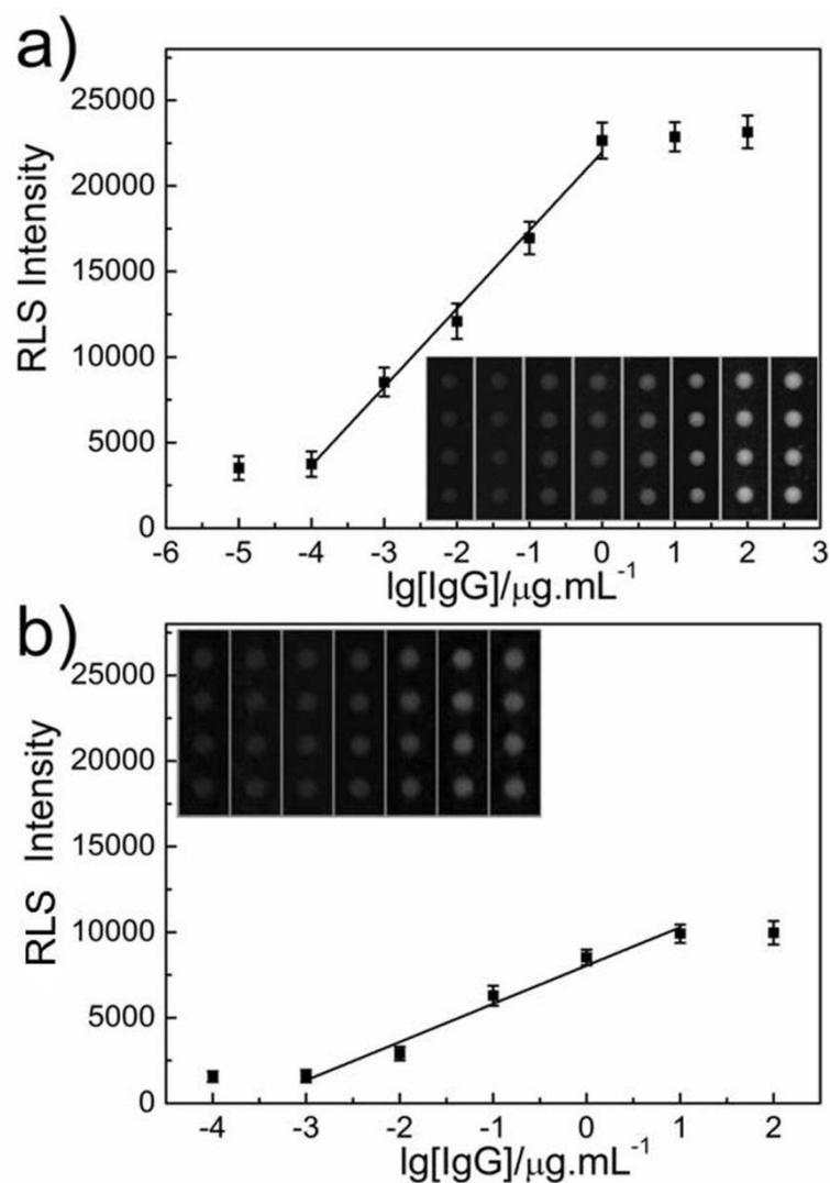
**Fig. S8.** Logarithmic plot of (a) PW-RLS scanner and (b) commercial scanner signal intensity as a function of the concentration of IgG in the probe solution. The insets were corresponding images of microarrays. The protein A concentration in the spotting solution was 100  $\mu\text{g/mL}$ .
