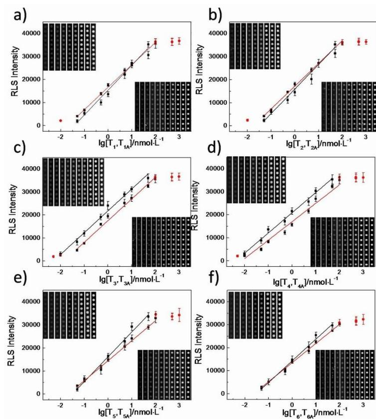
**Fig. S10.** RLS images and the corresponding logarithmic plots of the integrated RLS intensity as a function of the concentration of target ssDNAs  $T_n$  (●) and  $T_{nA}$  (■) in the solution. (a)-(f) represent 6 SNPs association for T2DM. The probe ssDNAs concentration in the spotting solution was 30  $\mu\text{M}$ . The target ssDNAs concentration in the solution was 0.01 nM, 0.05 nM, 0.1 nM, 0.5 nM, 1 nM, 5 nM, 10 nM, 50 nM, 100 nM, 500 nM and 1000 nM, respectively.
