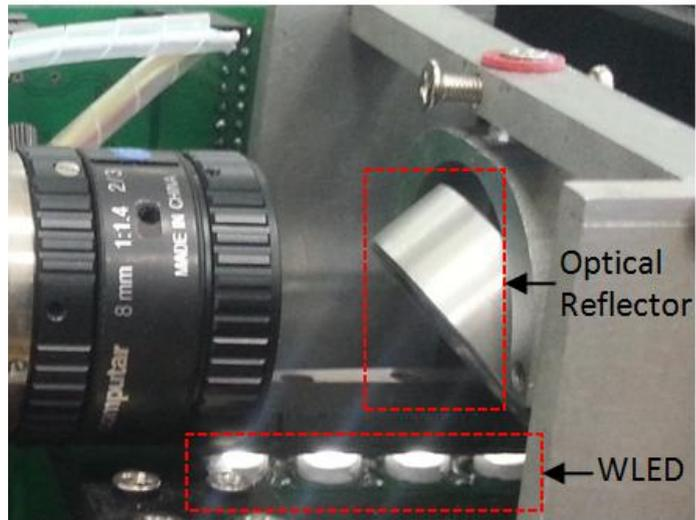
**Fig. S5.** The photograph of WLEDA assembled with optical reflector to generate the 90 ° folded imaging optical path.
