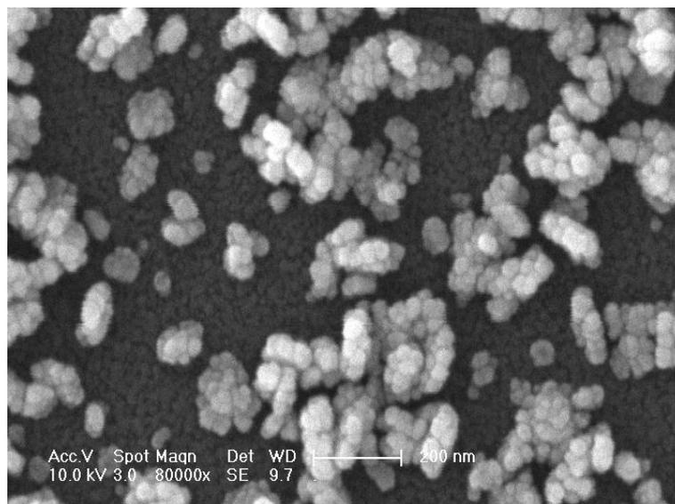
**Fig. S6.** Scanning electronic microscopy (SEM) micrographs of GNPs. The scale bar is 200 nm and the diameter of GNPs is about 60 nm.
