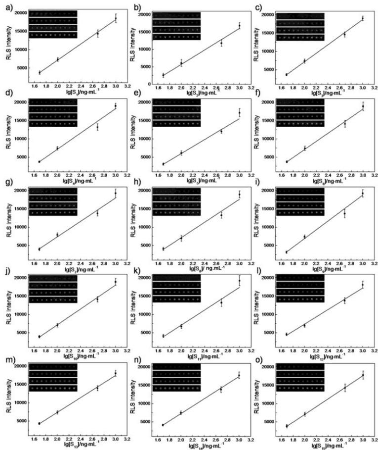
**Fig. S13.** RLS images and the corresponding logarithmic plots of the integrated RLS intensity as a function of the concentration of PCR products carrying rs6585205 amplified from genomic DNAs of (a)-(o) 15 T2DM patient blood samples. The concentrations of probe ssDNAs in the spotting solution were 30  $\mu$ M. The PCR product concentration was diluted to 1000 ng/mL, 500 ng/mL, 100 ng/mL and 50 ng/mL, respectively.
