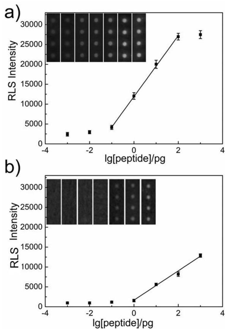
**Fig. S7.** Logarithmic plot of (a) PW-RLS scanner and (b) commercial scanner signal intensity as a function of the concentration of peptide on the microarray spots. The insets were corresponding images of microarrays.
