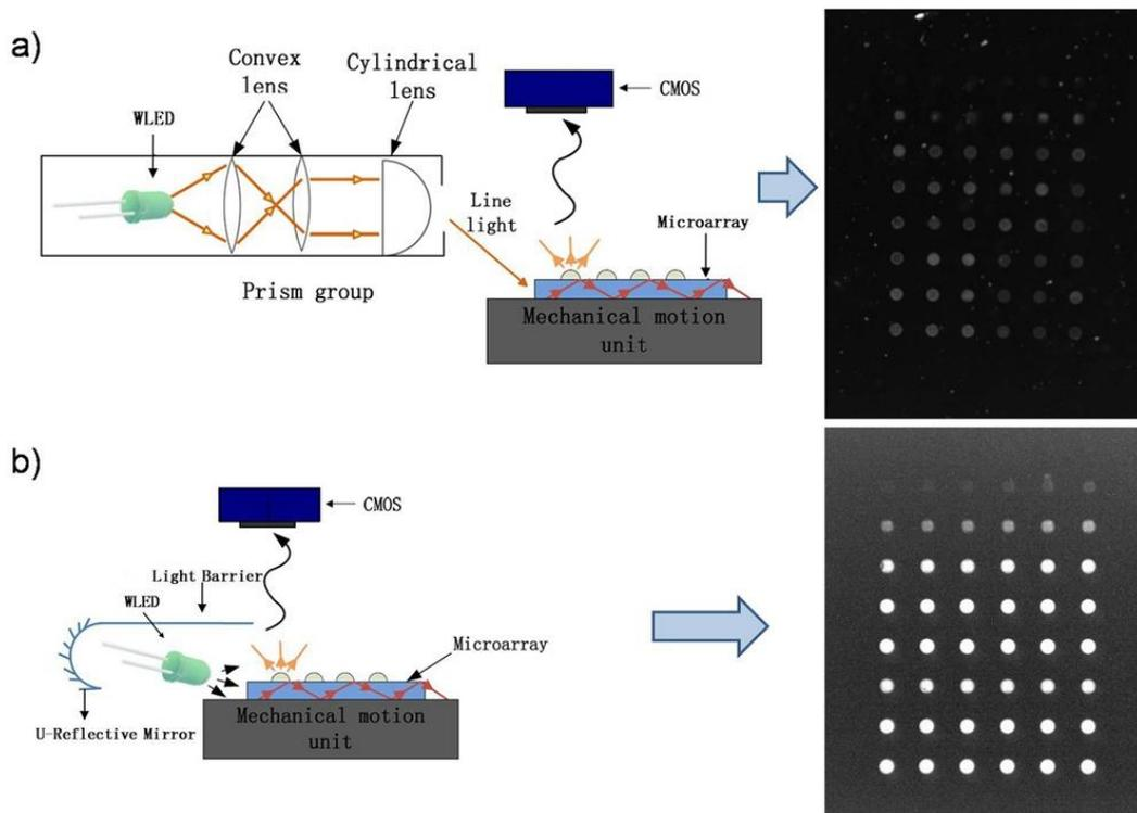
**Fig. S2.** RLS images and corresponding optical structure of PW-RLS scanner with (a) coupling lens and (b) U-reflective mirror and light barrier.
