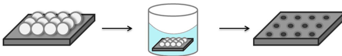
Fig. S2 Nanopores within a thin film of OTS prepared by particle lithography combined with solution immersion. 1 A drop of an aqueous suspension of silica mesospheres in water (10 \mu\text{L} ) was deposited on a clean Si(111) substrate. The sample was dried in air for 2 h to produce surface masks. As water evaporated during the drying step, capillary forces pull the mesospheres together to form crystalline layers on flat surfaces. The substrate was placed in an oven at 140 C overnight to temporarily anneal the mesospheres to the surface. After cooling, the sample was immersed in a 0.1% solution (v/v) of OTS in toluene for 5 h to form an OTS film surrounding the surface mask. To remove the mesoparticles, the substrate was sonicated for 15 min in ethanol and water successively. The sample was dried under argon before characterization with FMM-AFM.
