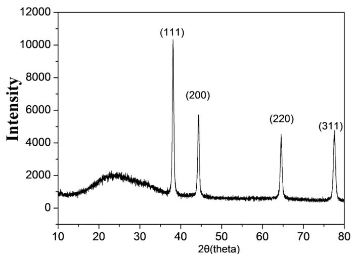
**Figure S9** X-ray diffraction spectrum of gold nanorods.
