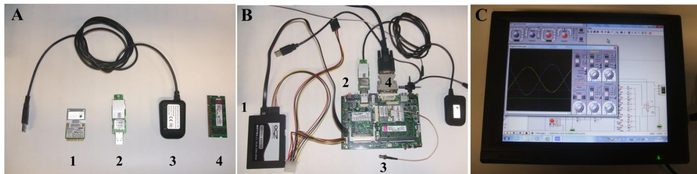
Fig. S2. Peripherals coupled to the CPU from the PG0004. In A, 1: Bluetooth and Wi-Fi wireless board, 2: 3G modem for GPRS communication, 3: GPS receiver, and 4: RAM memory. In B are shown the peripherals in A that were connected to the CPU, and 1: HD, 2: CPU, 3: wireless antenna, 4: VGA output for touchscreen monitor presented in C.
