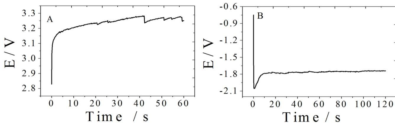
Fig. S5. Chronopotentiometric curves applied in the anodic (A) and cathodic pre-treatments (B) of the BDD electrode using the PG004. In (A)  $50 \text{ mA cm}^{-2}$  was applied for 60 s, and (B)  $-50 \text{ mA cm}^{-2}$  for 120 s in  $0.1 \text{ mol L}^{-1} \text{ H}_2\text{SO}_4$  as supporting electrolyte.
