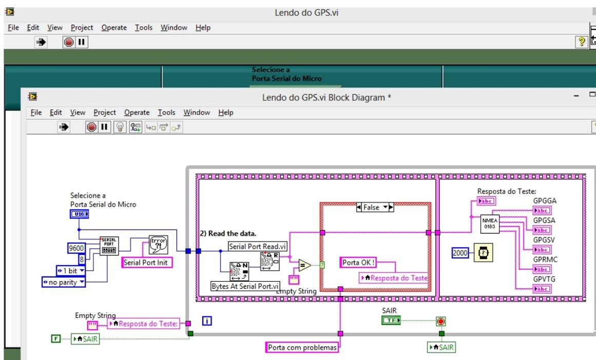
Fig. S9. Receiving data via GPS. Data in the NMEA navigation protocol using the COM4 serial port from the CPU of the PG004 (A). Block diagram of the program developed in LabView (B).
