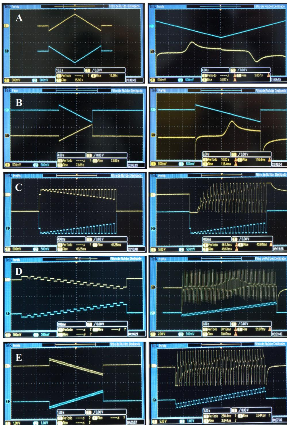
Fig. S4. Tests performed using the PAR model 173A and the oscilloscope employing the developed software. Applied potential (blue curves) and the potential available in the electrochemical cell (yellow curves), and the generated current (yellow curves) are shown. From A to E are presented the voltammograms from: cyclic, linear, normal pulse, differential pulse, and square wave.
