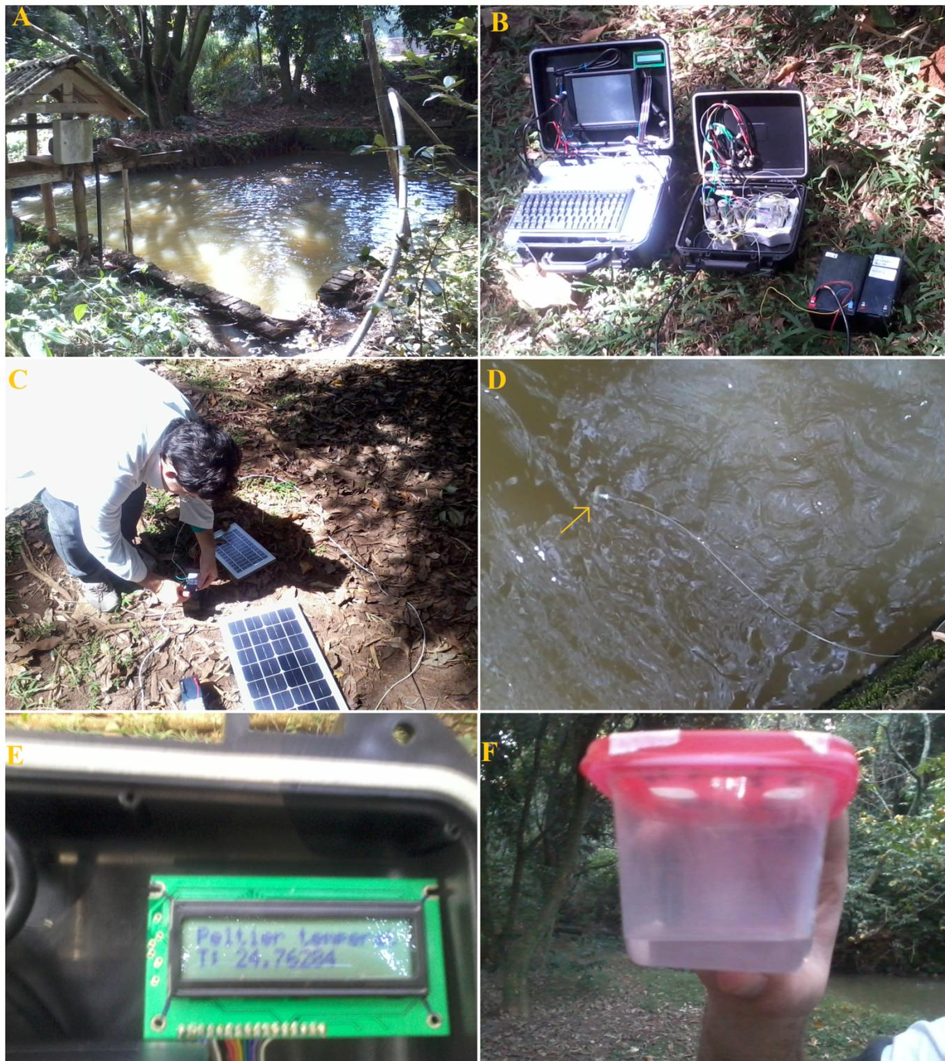
Fig. S8. *In situ* analysis using the PG004. (A) Dam of Monjolinho Lake, (B) a photograph of PG004, and extra batteries (C) being recharged employing the solar boards. In (D), the sample being collected and in-line filtered (indicated by the arrow) using a 0.45  $\mu\text{m}$  filter is shown. The real temperature of the sample onto the EFC by using the thermostated control driven by the microcontrolled board developed (E). Waste bottle (F).
