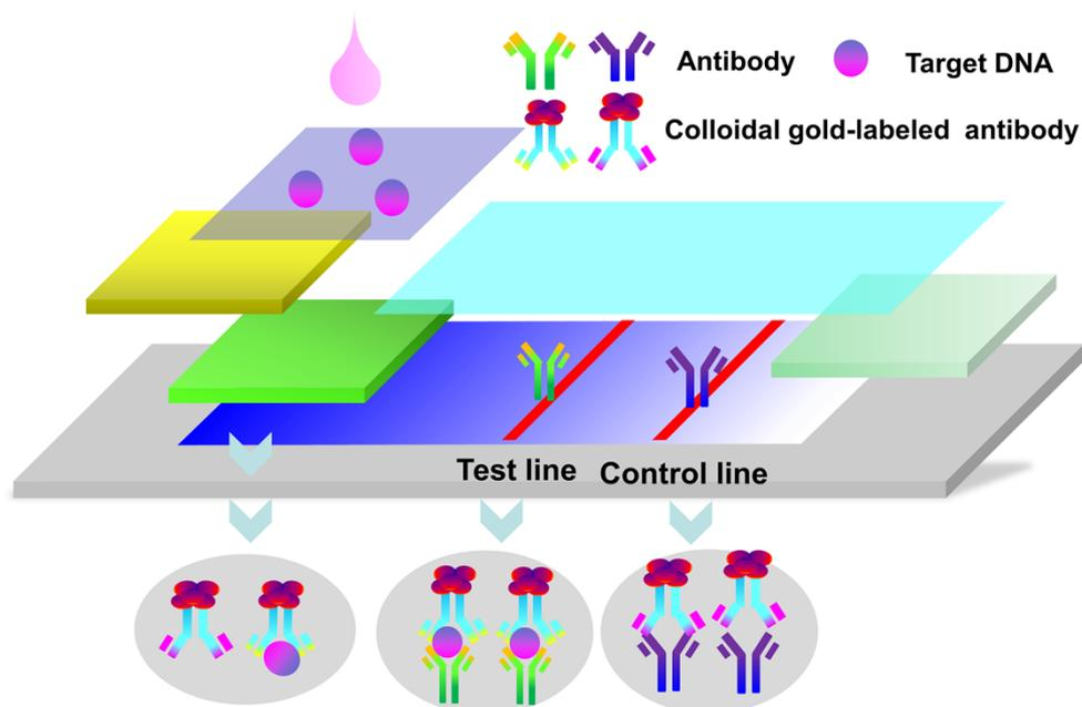
**Figure S6** Principle of lateral-flow dipstick (LFD)
