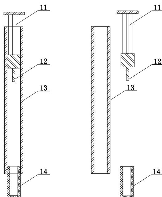
**Figure S3** The assembly and exploded view of “injector” cartridge. Number 11, syringe piston; 12, small bulge part of the syringe piston; 13, syringe outer tube wall; 14, reaction tube. The reaction tube inner diameter and height are respectively 3 mm and 15 mm.
