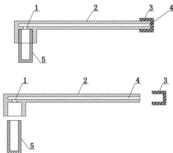
**Figure S1** The assembly and exploded view of the non-oil sealed LFD cartridge. Number 1, interconnecting orifice; 2, detection container; 3, end cap; 4, Cavity for LFD strip; 5, reaction tube. The diameter of the interconnecting hole is 1.5 mm. The reaction tube inner diameter and height
