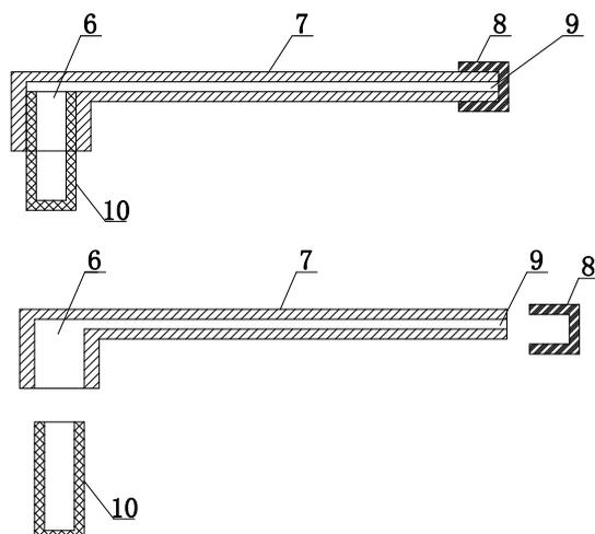
**Figure S2** The assembly and exploded view of horizontal type cartridge. Number 6, interconnecting hole; 7, detection container; 8, end cap; 9, LFD container; 10, reaction tube. The reaction tube inner diameter and height are respectively 3 mm and 15 mm.
