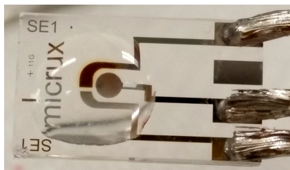
Fig. S6. Photo taken of a Pt TFE with 30 % m_{PMMA}/m_{Tot.} PMMA- [C_2mim][NTf_2] electrolyte after long-term scanning in the presence of 100 % vol. O_2 flow. Sign of accumulation of counter electrode reaction product on the CE and WE is clearly visible.
