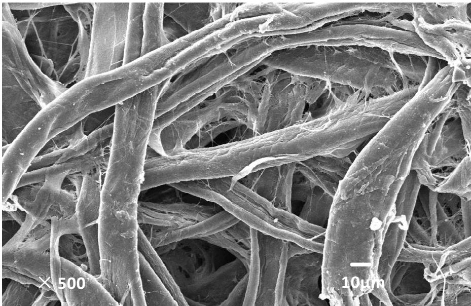
**Fig. S-2** SEM image of commercially available filter paper.
