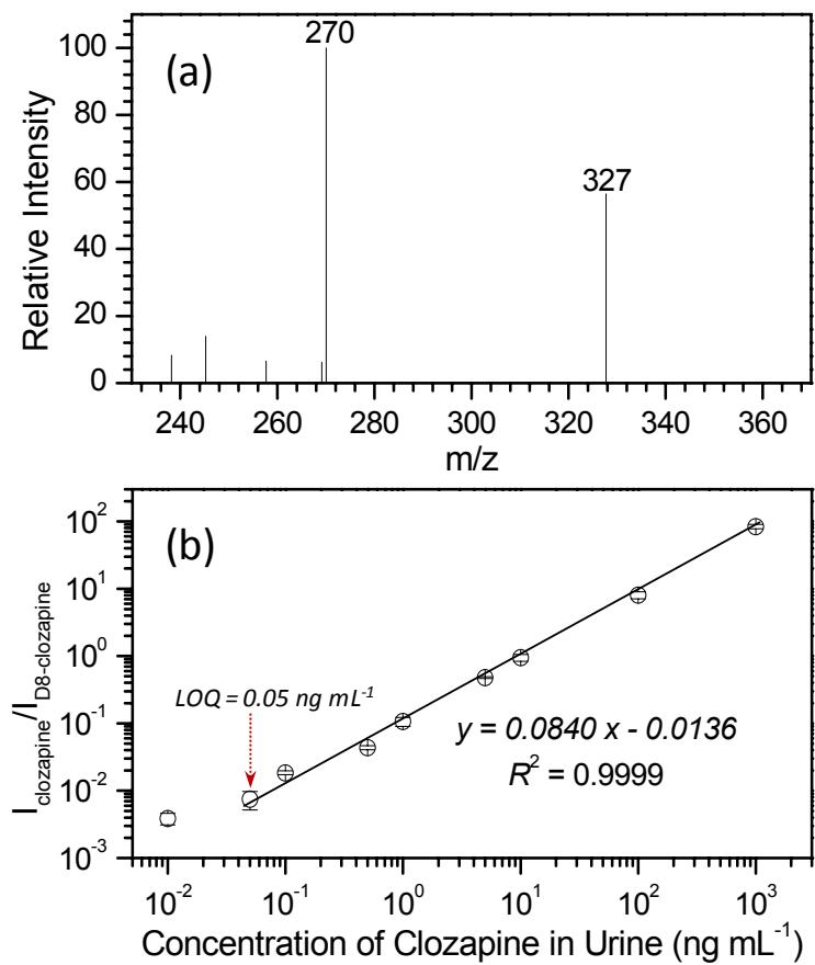
**Fig. S-5** (a) MS/MS spectrum for  $10 \text{ ng mL}^{-1}$  clozapine in  $2.0 \mu\text{L}$  raw urine using silica coated paper for paper spray. (b) Quantitation analysis of raw urine spiked clozapine ( $0.01 - 1,000 \text{ ng mL}^{-1}$ ) and its isotopomer  $[\text{D}_8]\text{clozapine}$  ( $10 \text{ ng mL}^{-1}$ ). The analysis was carried out by applying  $3.5 \text{ kV}$  DC voltage and  $20 \mu\text{L}$  acetonitrile.
