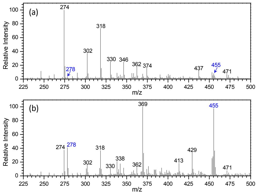
**Fig. S-3** Full mass spectrum of dried blood spot containing  $1\mu\text{g mL}^{-1}$  amitriptyline ( $m/z$  278) and verapamil ( $m/z$  455) by using (a) commercially available filter paper and (b) silica coated paper. Acetonitrile was used as the spray solvent, and spray voltage of 3.5 kV was applied for paper spray.
