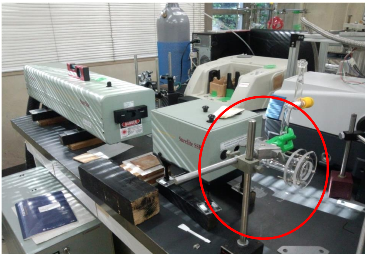
Figure S7. Overview of the reaction apparatus for Cl• capturing experiments by DPPH• in the gas phase.
