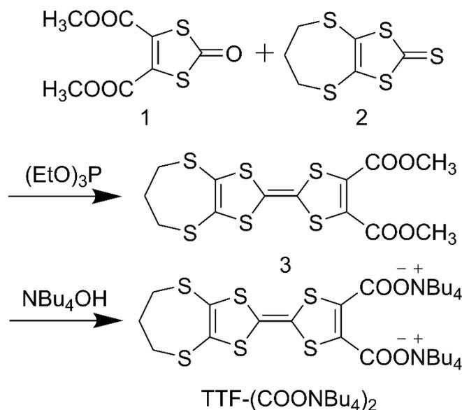
Figure S1. Synthetic procedures of TTF-(COONBu<sub>4</sub>)<sub>2</sub>.
