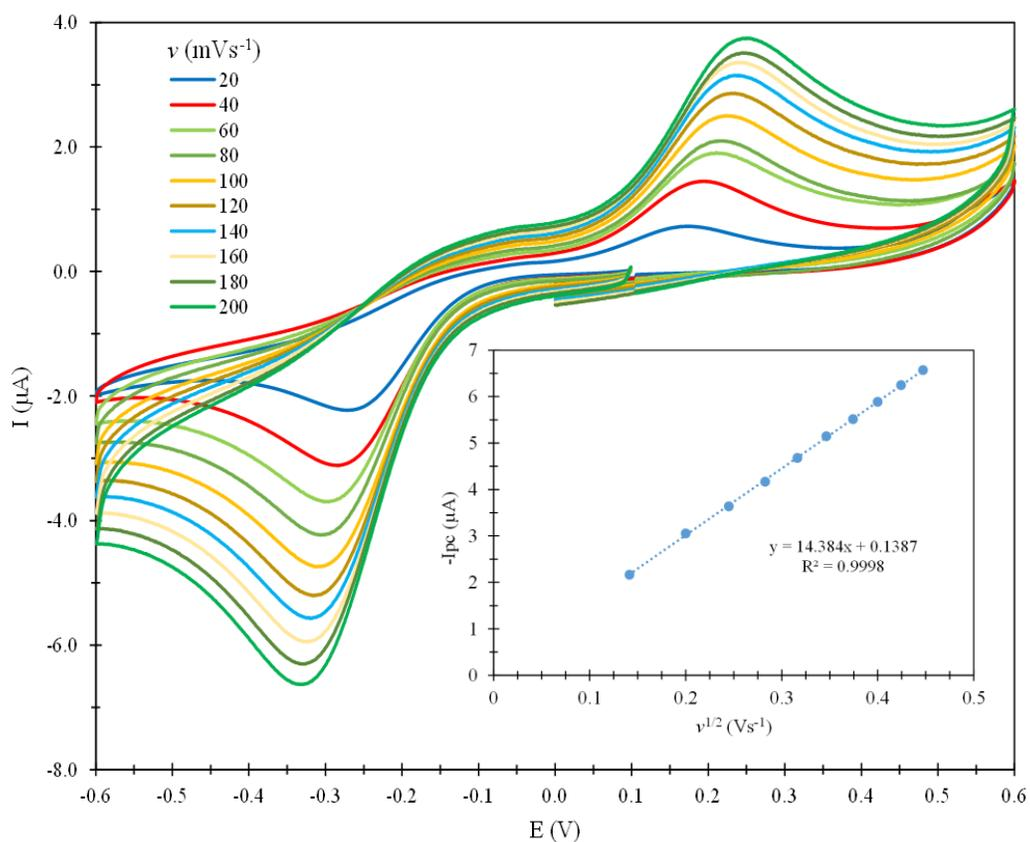
**Figure S1.** Family of cyclic voltammograms recorded in the system SPE / quinone, Q, 100  $\mu\text{M}$ , acetates buffered 0.1M at pH  $4.70 \pm 0.01$  and  $(30.0 \pm 0.5)^\circ\text{C}$ , considering different potential scan rates, indicated in the figure. The inset shows the variation of the cathodic peak's current as a function of the square root of the scan rate.
