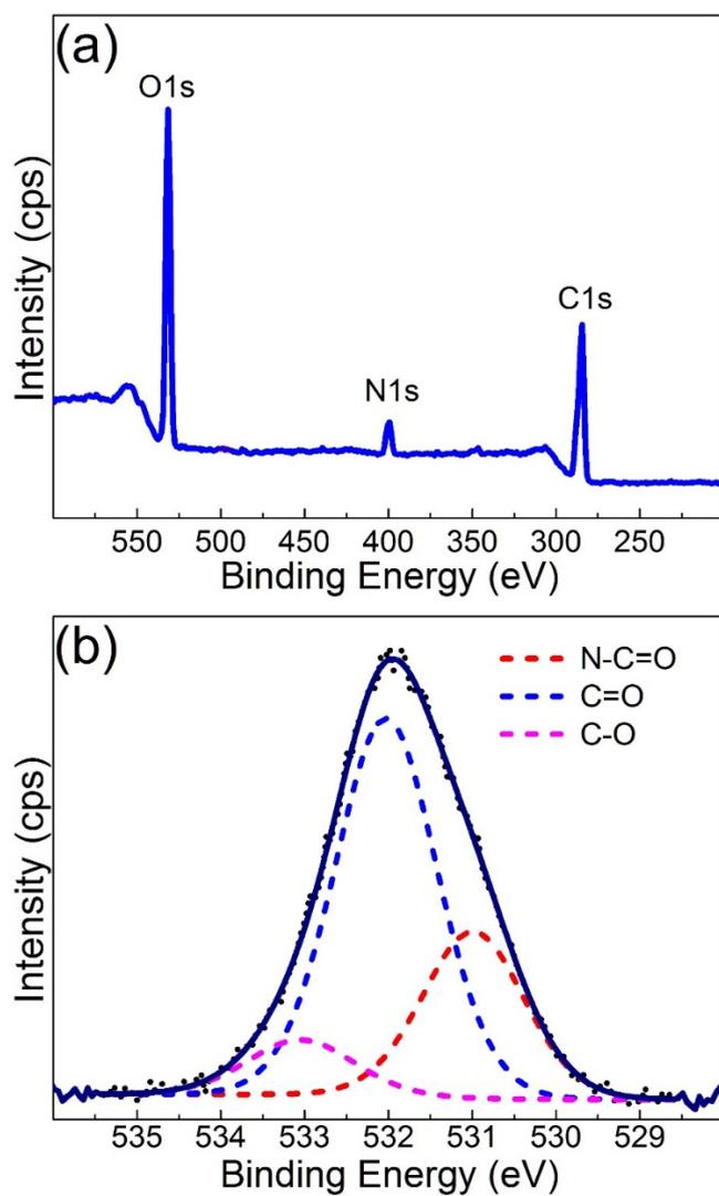
**Fig. S2.** XPS (a) survey and (b) O1s spectra of A-CDs
