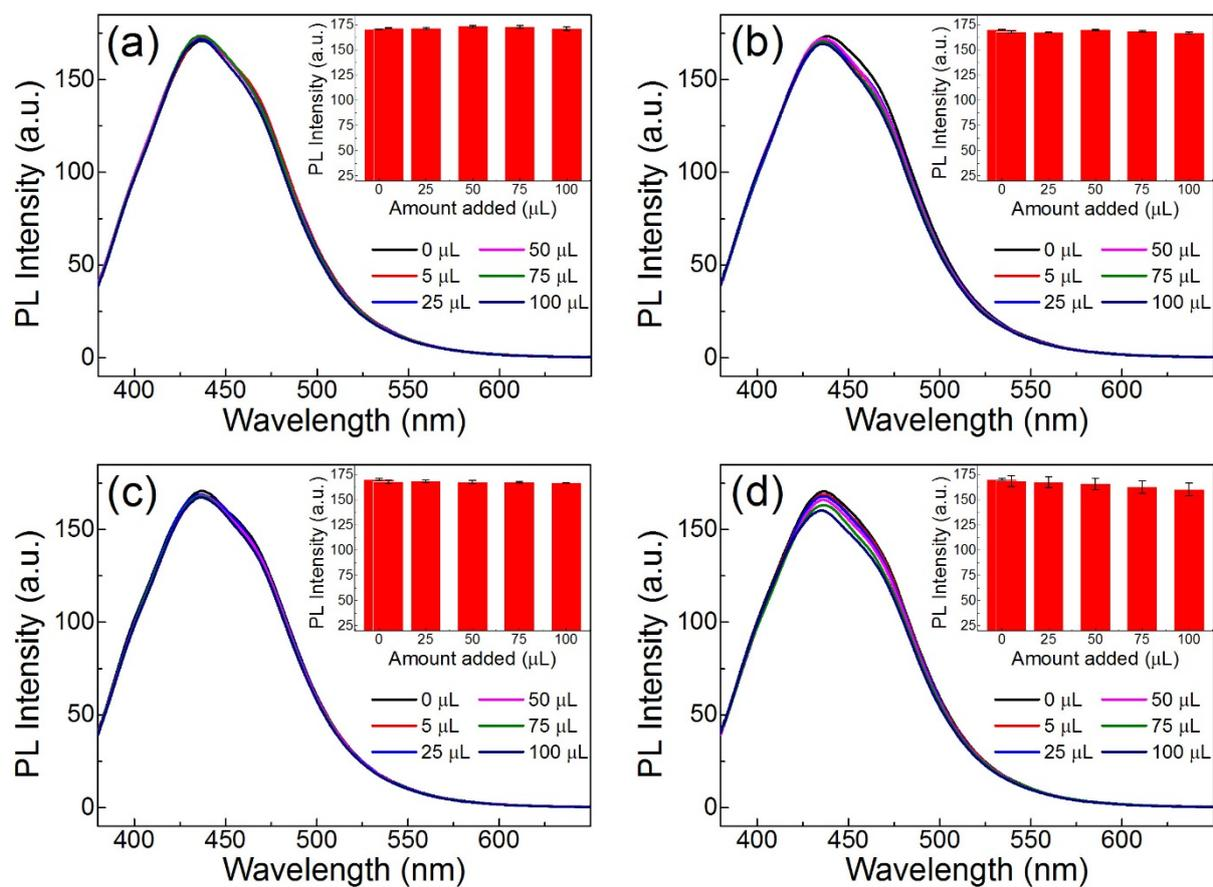
**Fig. S6.** Photoluminescence responses of A-CDs against (a) acetone, (b) ethanol, (c) methanol and (d) propylene glycol (1,2-propanediol)
