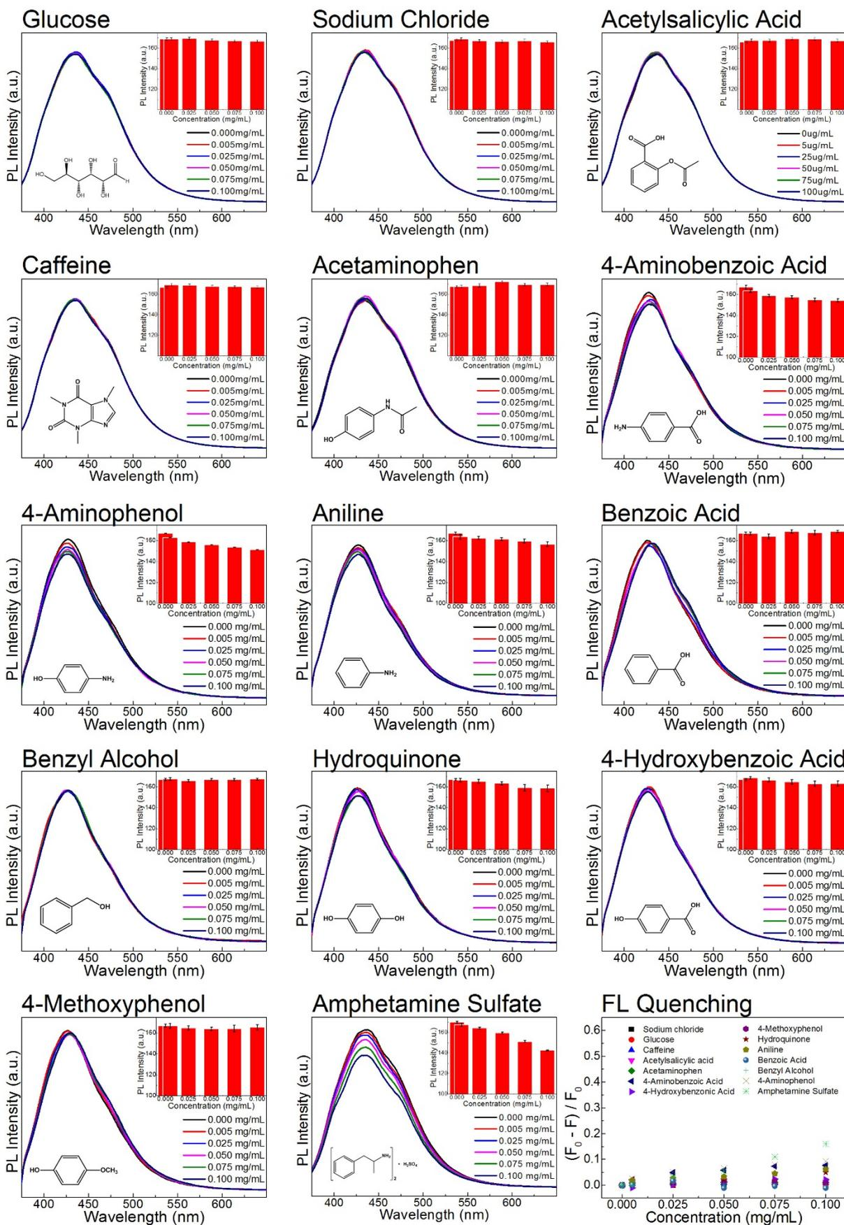
**Fig. S7.** Photoluminescence spectra and quenching of other molecules tested
