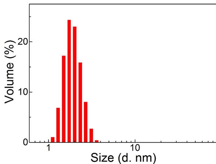
**Fig. S1.** Hydrodynamic size of A-CDs measured by DLS
