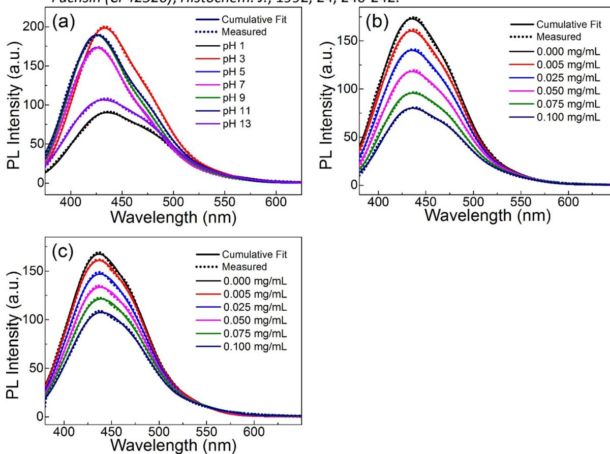
**Fig. S5.** Measured photoluminescence intensity and cumulative fitting spectra of (a) pH effects, (b) PAC-diol and (c) P2P samples
