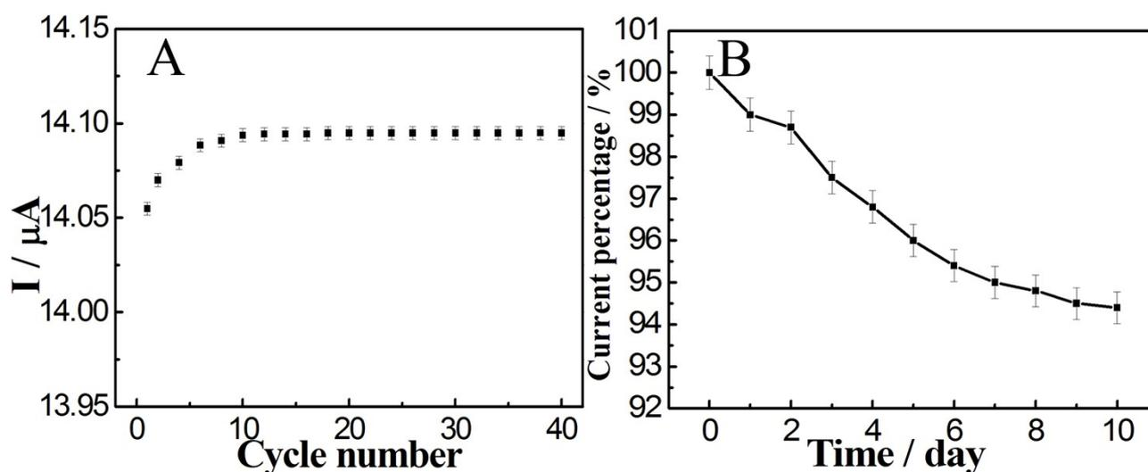
**Fig. S4.** (A) Peak current response of 4-amino thiophenol/AuNPs/GOD-HRP/MUA-MCH/Au electrode for forty continuous scanning in 0.2 M PBS + 5 mM  $\text{K}_3\text{Fe}(\text{CN})_6$  at  $100 \text{ mV s}^{-1}$ . (B) The peak current response of 4-amino thiophenol/AuNPs/GOD-HRP/MUA-MCH/Au electrode in 0.2 M PBS + 5 mM  $\text{K}_3\text{Fe}(\text{CN})_6$  at  $100 \text{ mV s}^{-1}$  for 10 days.
