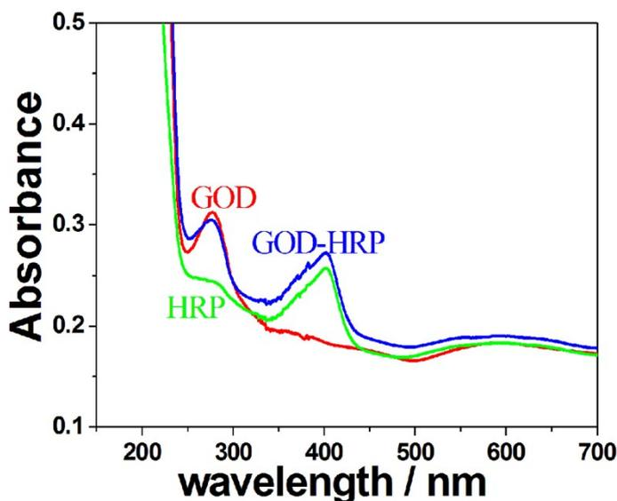
**Fig. S2.** UV-Vis spectra of GOD (red line), HRP (green line) and GOD-HRP (blue line) on the transparent quartz glass substrate.
