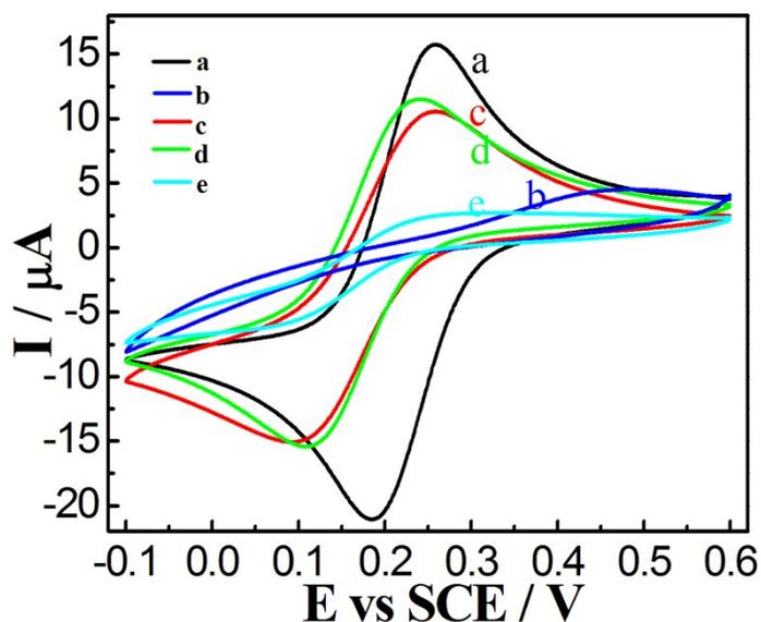
**Fig. S3.** CVs of the Au (curve a, black line), MUA-MCH/Au (curve b, blue line), GOD-HRP/MUA-MCH/Au (curve c, red line), AuNPs/GOD-HRP/MUA-MCH/Au (curve d, green line) and 4-amino thiophenol/AuNPs/GOD-HRP/MUA-MCH/Au electrode (curve e, cyan line) in 0.2 M PBS + 5 mM  $\text{Fe}(\text{CN})_6^{3-/4-}$  + 10 mM glucose at  $100 \text{ mV s}^{-1}$ .
