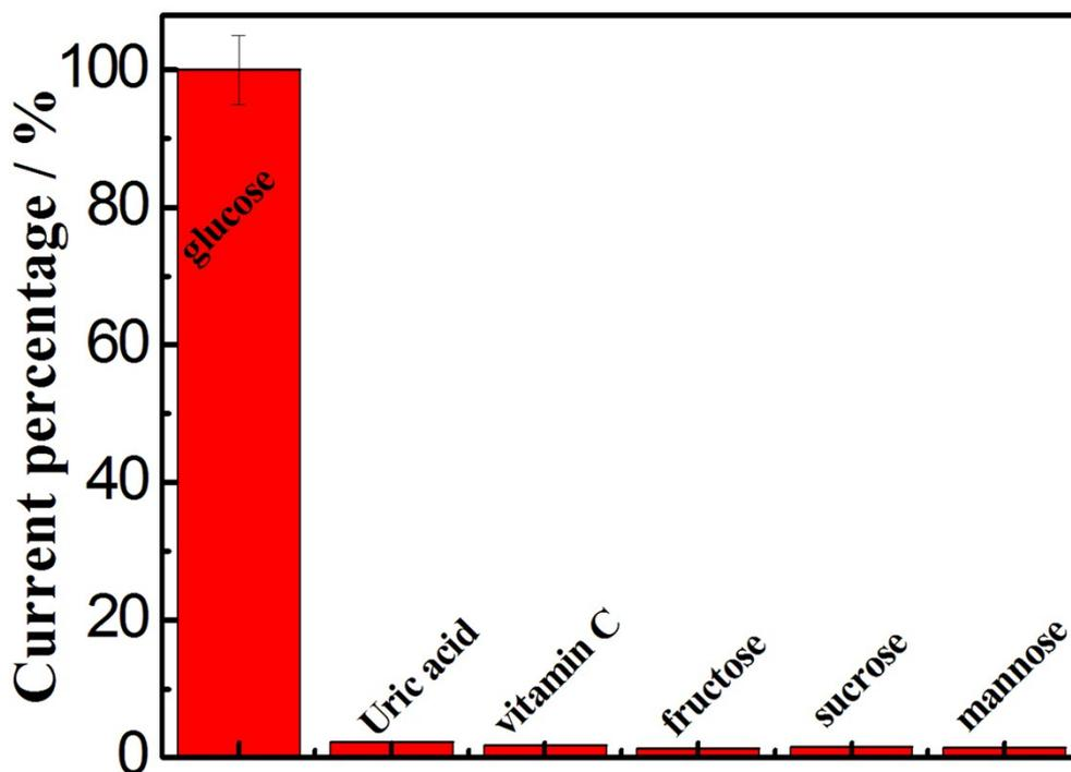
**Fig. S5.** Selectivity test of the new developed biosensor in 0.2 M PBS (pH 7.0) + 5 mM  $K_3Fe(CN)_6$  in the presence of 2 mM glucose, or 6.0 mM uric acid, or 6.0 mM vitamin C, or 6.0 mM fructose, or 6.0 mM sucrose or 6.0 mM mannose.
