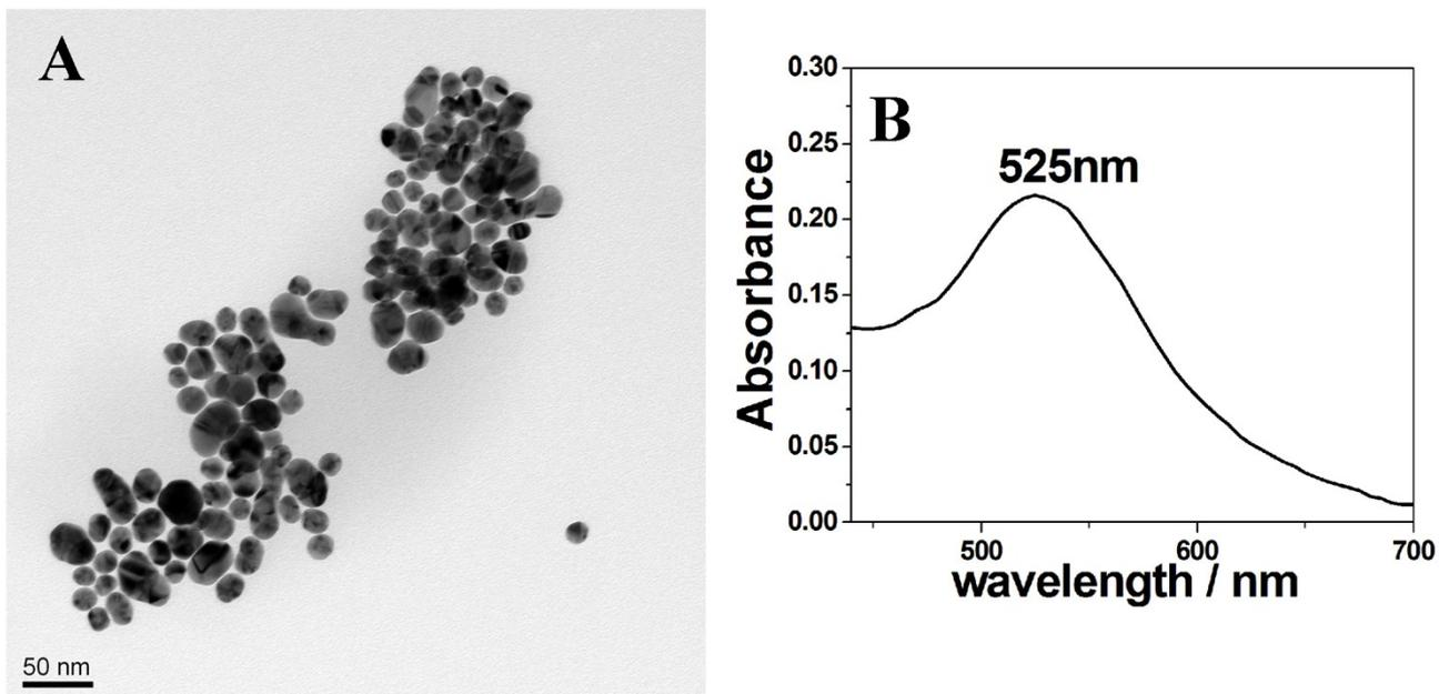
**Fig. S1.** TEM image (A) and UV-Vis absorption spectroscopy (B) of prepared AuNPs.
