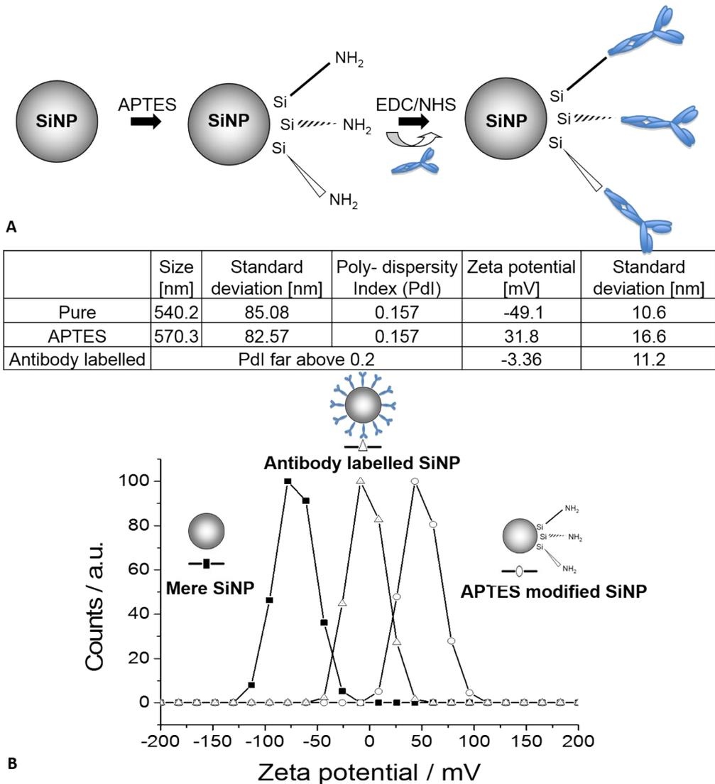
**Fig. 1S** A) Schematic overview of the SiNP modification. B) DLS and Zeta potential measurement profiles demonstrate that DLS and Zeta potential measurement can be successfully used to monitor the surface modification.
