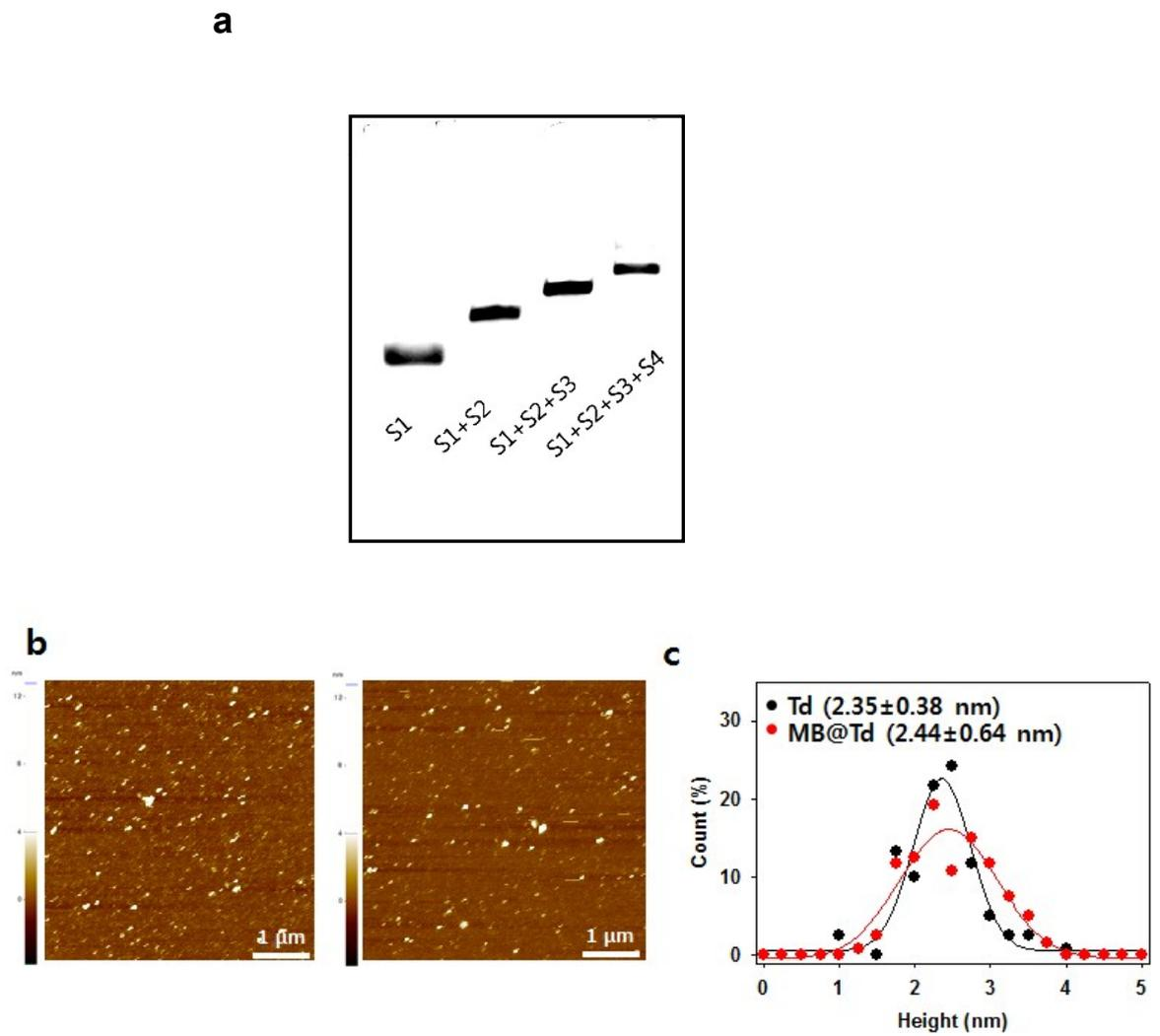
**Fig. S1.** (a) Native PAGE (6%) to verify assembly of Td. (b) AFM images of Td (left) and MB-loaded Td (right) showing the dried state of nanoparticles. (c) The averaged heights of Td (black) and MB@Td (red) were estimated from 120 representative particles in AFM images.
