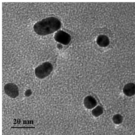
**Figure S3.** HRTEM image of the Au/GQDs composites.
