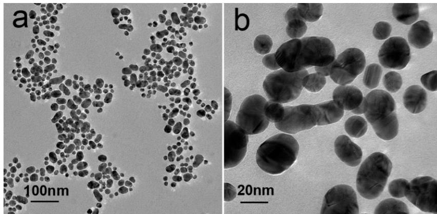
**Figure S2.** TEM images of Au nanoparticles.
