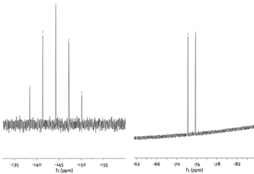
**Figure S7.** Partial  $^{31}\text{P}$  NMR spectrum ( $\text{CD}_3\text{CN}$ , 243 MHz) of  $2\cdot\text{PF}_6$  isolated from the bulk photolysis experiment (left) and  $^{19}\text{F}$  NMR spectrum ( $\text{CD}_3\text{CN}$ , 471 MHz) of the same salt (right).
