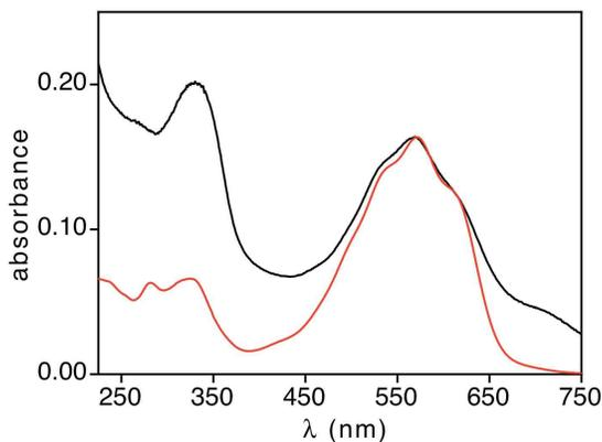
**Figure S6.** Normalized UV-vis absorption spectra of a  $\text{CH}_3\text{CN}$  solution of  $\mathbf{2} \cdot \text{PF}_6$  isolated from the bulk photolysis experiment (black line) and the spectrum that results when a wet  $\text{CH}_3\text{CN}$  solution (5% v/v  $\text{H}_2\text{O}$ ) of **1o** is irradiated with 365 nm light for 2200 s (red line).
