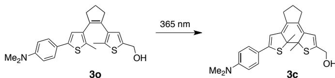
**Ring-closing of 1-(2-hydroxymethyl-5-methylthien-3-yl)-2-(2-(4-(dimethylamino)phenyl)-5-methylthien-3-yl)cyclopentene (**3o**).** A CH<sub>3</sub>CN solution of **3o** was irradiated with 365 nm light until all changes in the UV-vis spectra stopped. The red solution contained 82% of the ring-closed isomer as measured by <sup>1</sup>H NMR spectroscopy.
