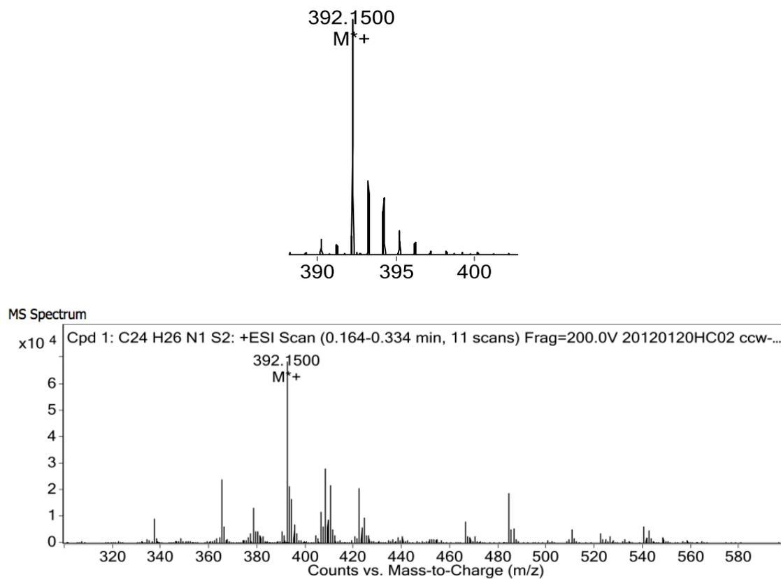
**Figure S8.** ESI-(+) HRMS analysis of  $2\cdot\text{PF}_6$  isolated from the bulk photolysis experiment. The full analysis is shown at the bottom.
