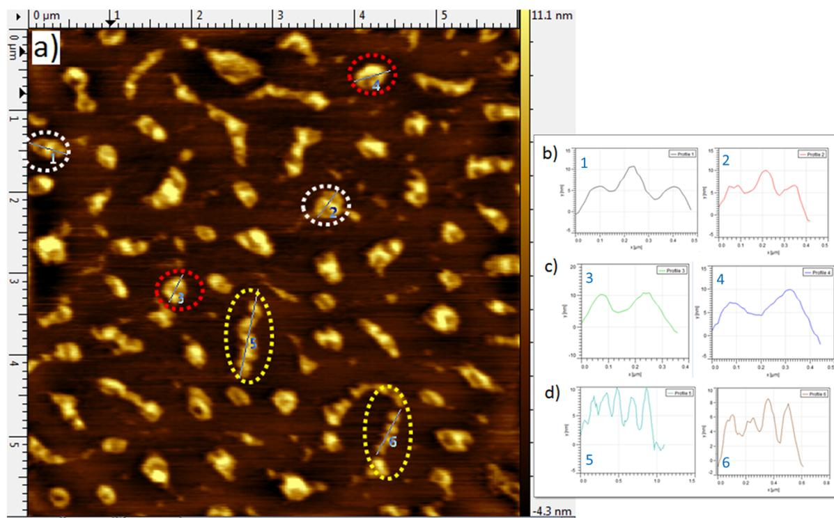
**Figure S9.** (a) AFM topography image of PS catenanes (**6**) on a  $6 \times 6 \mu\text{m}$  scale on mica, line profile of the representative samples of (b) PS-[2]catenanes, (c) cyclic isomer of PS, and (d) PS-[ $n$ ]catenanes ( $n \geq 3$ ).
