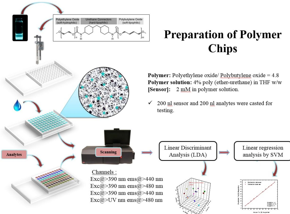
**Figure 1.** Procedure of preparation of polymer chips
