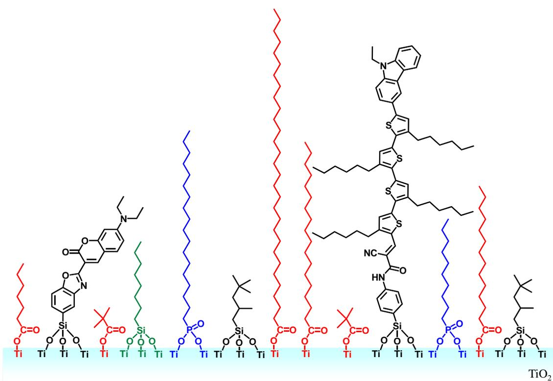
**Fig. S3** Schematic drawing of the ‘alkyl-thicket’ structure on the **ADEKA-1** + **SFD-5**-co-adsorbed  $\text{TiO}_2$  electrode formed by the hierarchical multi-capping treatment.
