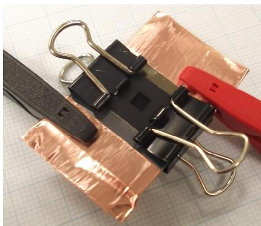
**Fig. S5** Schematic drawings of the square shade mask and the TiO<sub>2</sub> film with the sensitizing dyes and a photograph of the electrochemical cell of the open sandwich type used in this work. In the photovoltaic measurements, the spaces between the shade mask and the Cu conduction tapes were also shaded to avoid light scatter and other undesirable effects producing uncertainties in the measurements.
