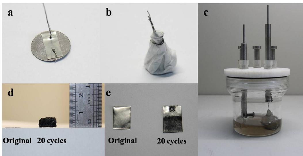
Figure S1 The experimental photographs of (a) cathode: carbon paper fixed by molybdenum sheets and wire, (b) cathode wrapped by glass fiber, (c) sealed teflon electrolytic tank, (d) the comparison of carbon paper: original (left) and discharged for 20 cycles (right) and (e) the comparison of aluminium foil: original (left) and discharged for 20 cycles (right).
