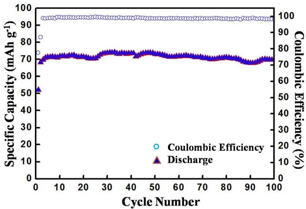
Figure S2 Cycle performance and coulombic efficiency of Al-ion full battery at the current density of 100 mA g<sup>-1</sup>.
