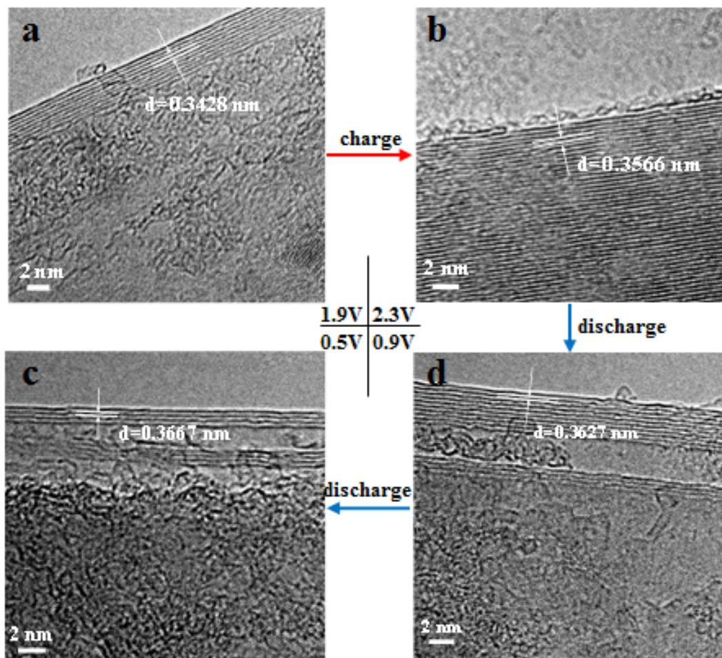
Figure S3 HRTEM images of the products after charge (a,b) and discharge (c,d) processes.
