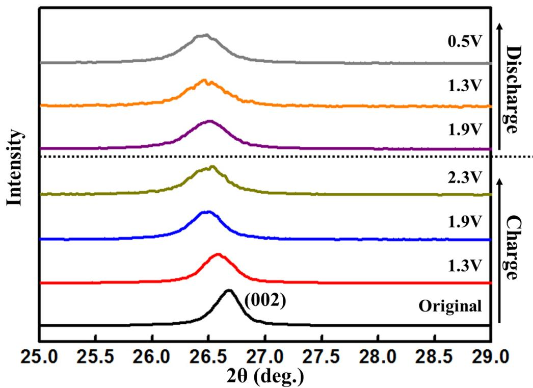
Figure S4 The XRD patterns of the products through a charge-discharge cycle.
