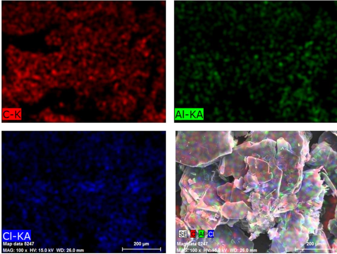
Figure S5 EDS mapping images of the charged cathode.
