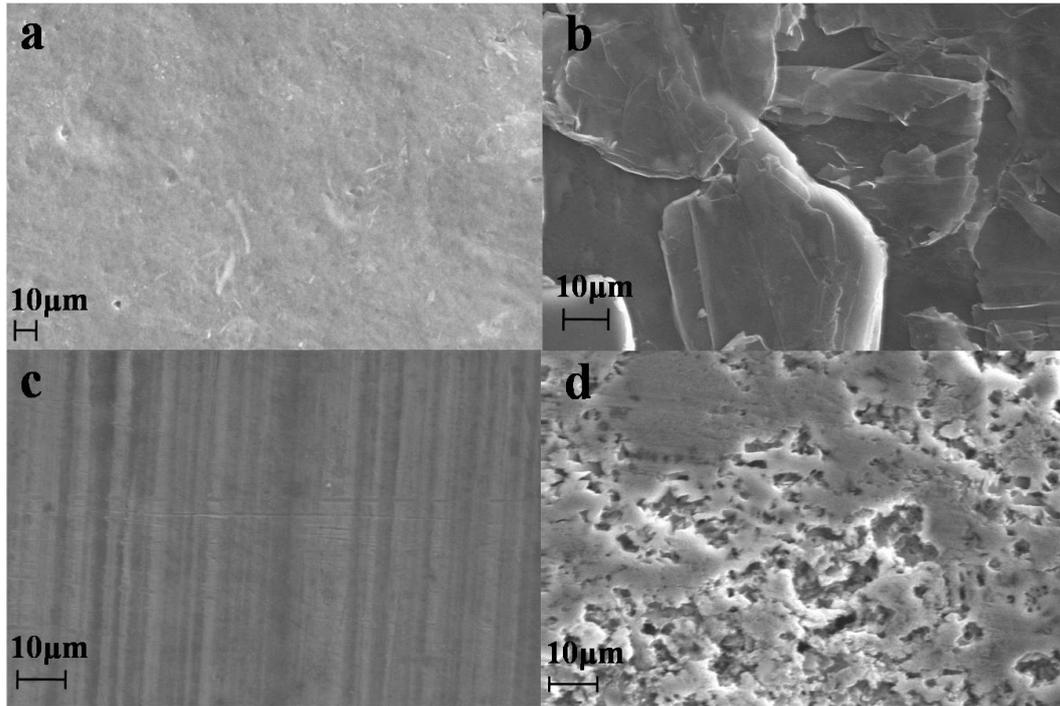
Figure S6 SEM images of (a) original carbon paper, (b) carbon paper after 20 cycles, (c) original aluminium foil and (d) aluminium foil after 20 cycles.
