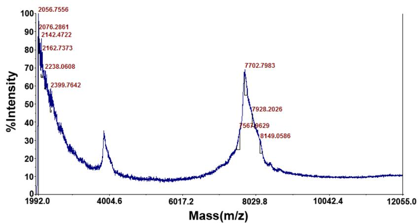
Fig. S2: The MALDI-TOF-MS of ON623-Ce6 Conjugates was carried out on an ABI 4800 MALDI-TOF with 2',4',6'-Trihydroxyacetophenone monohydrate (THAP) as matrix.
