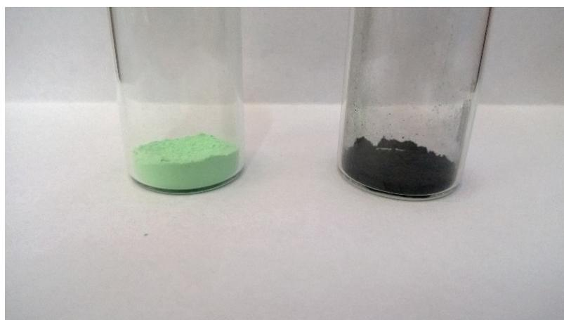
**Figure S4** Photograph of the Ni(OH)<sub>2</sub> (left) and Ni(OH)<sub>2</sub>@PPy (right). As the green powder turn to black after PPy coating process, indicating the successful encapsulation of PPy onto the Ni(OH)<sub>2</sub> surface.
