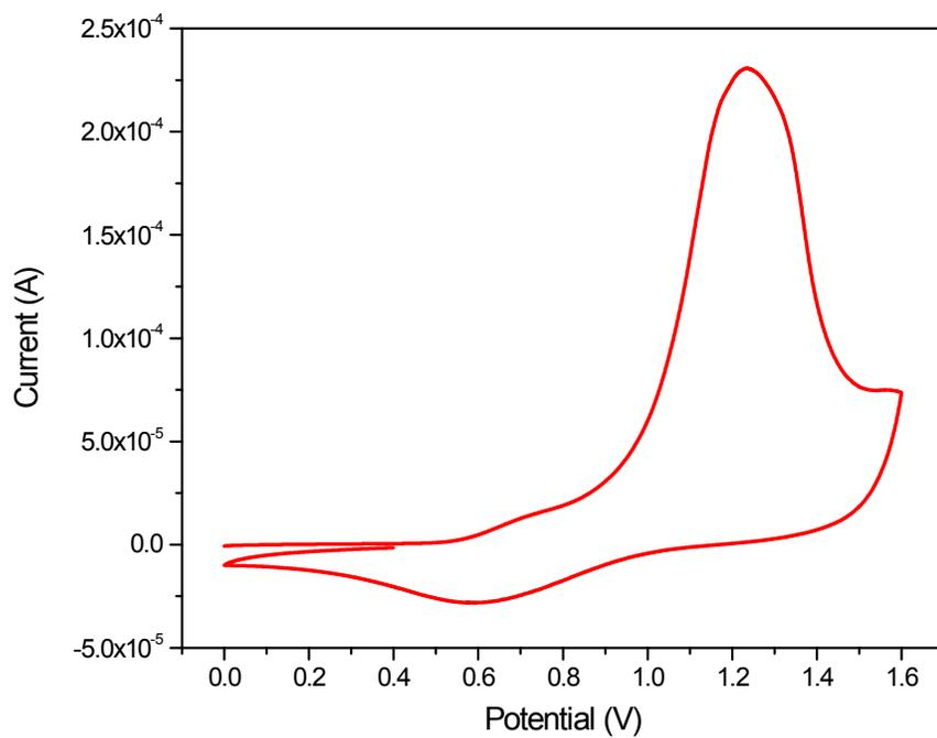
**Fig. S17** The oxidation cyclic voltammogram of a **P2** thin film at a scan rate of  $0.100 \text{ V s}^{-1}$ .
