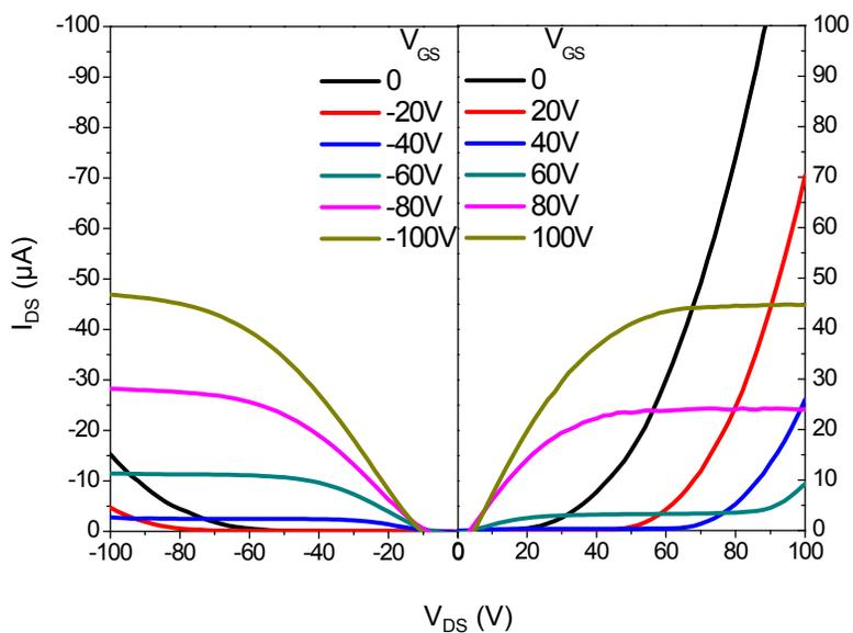
**Fig. S14** Output curve of an OTFT device based on a thin film of **P2** annealed at 200 °C.
