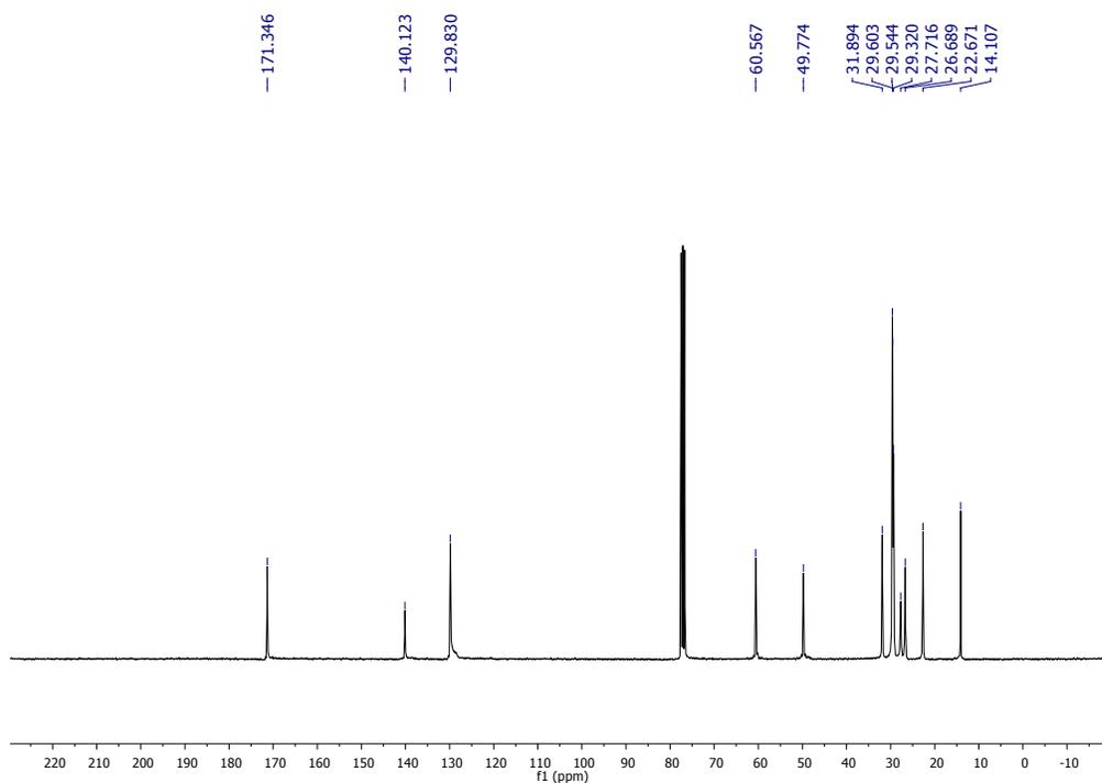
**Fig. S10** 75 MHz  $^{13}\text{C}$  NMR spectrum for *N,N'*-(1,4-phenylene)bis(*N*-dodecyl-2-hydroxyacetamide) (**2**) in chloroform-*d*.
