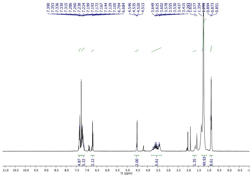
**Fig. 6** 300 MHz  $^1\text{H}$  NMR spectrum for 1,5-didodecyl-3,7-bis(phenylthio)-5,7-dihydropyrrolo[2,3-*f*]indole-2,6(1*H*,3*H*)-dione (**3**) in chloroform-*d*.
