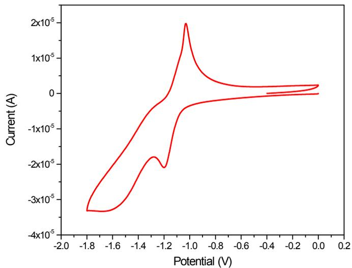
**Fig. S16** The reduction cyclic voltammogram of a **P2** thin film at a scan rate of  $0.100 \text{ V s}^{-1}$ .
