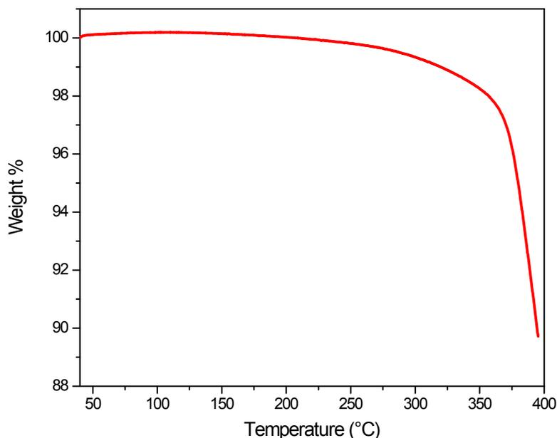
**Fig. S20** TGA curve of **P2** under nitrogen at a heating rate of 10 °C min<sup>-1</sup>.
