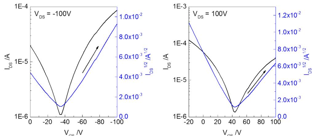
**Fig. S13** Transfer curve of an OTFT device based on a thin film of **P2** annealed at 200 °C
