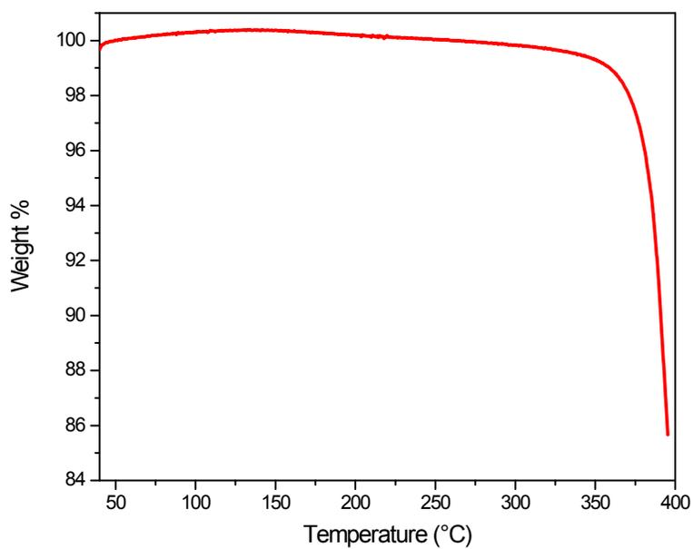
**Fig. S19** TGA curve of **P1** under nitrogen at a heating rate of 10 °C min<sup>-1</sup>.
