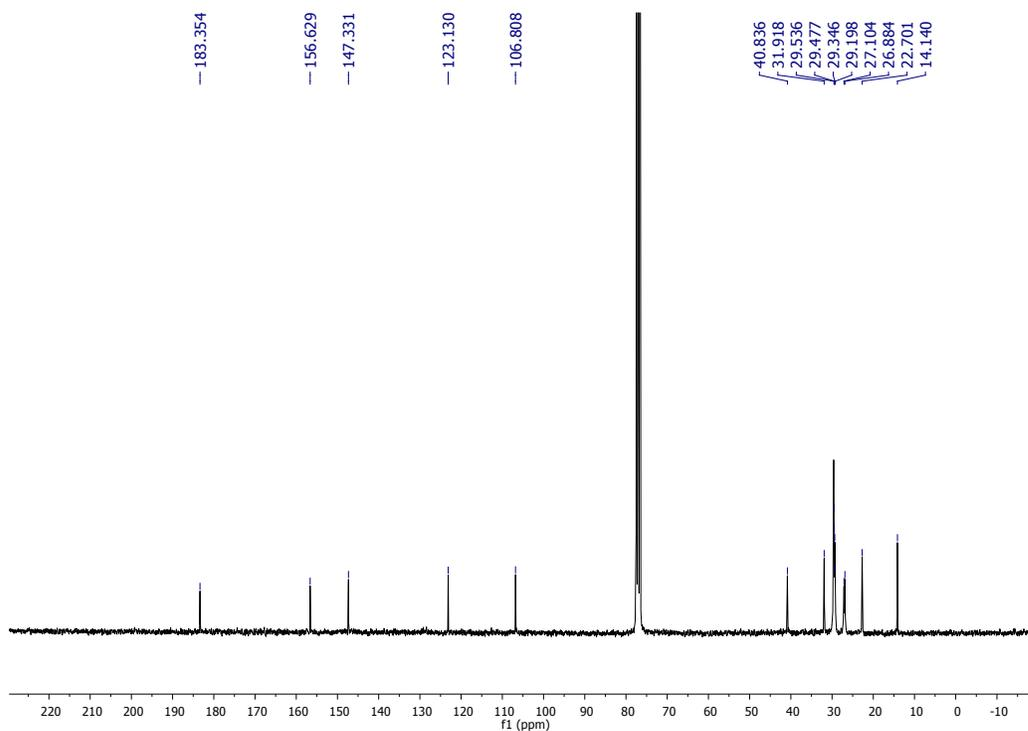
**Fig. S11** 75 MHz  $^{13}\text{C}$  NMR spectrum for 1,5-didodecylpyrrolo[2,3-*f*]indole-2,3,6,7(*1H,5H*)-tetraone (**4**) in chloroform-*d*.
