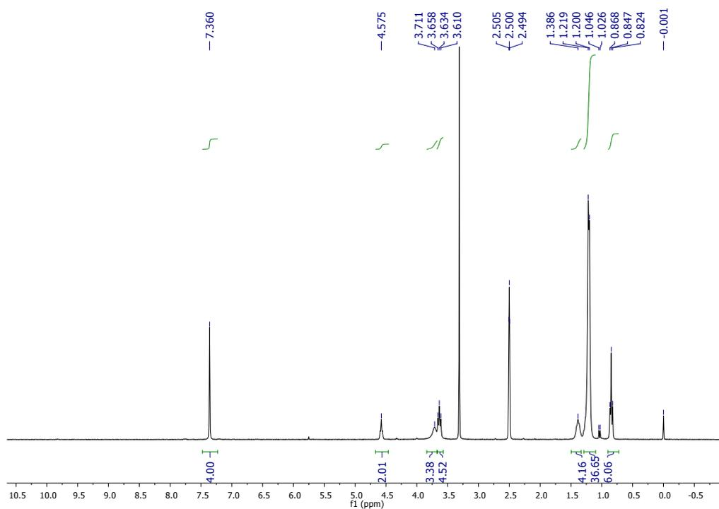
**Fig. S5** 300 MHz  $^1\text{H}$  NMR spectrum for *N,N'*-(1,4-phenylene)bis(*N*-dodecyl-2-hydroxyacetamide) (**2**) in DMSO- $d_6$ .
