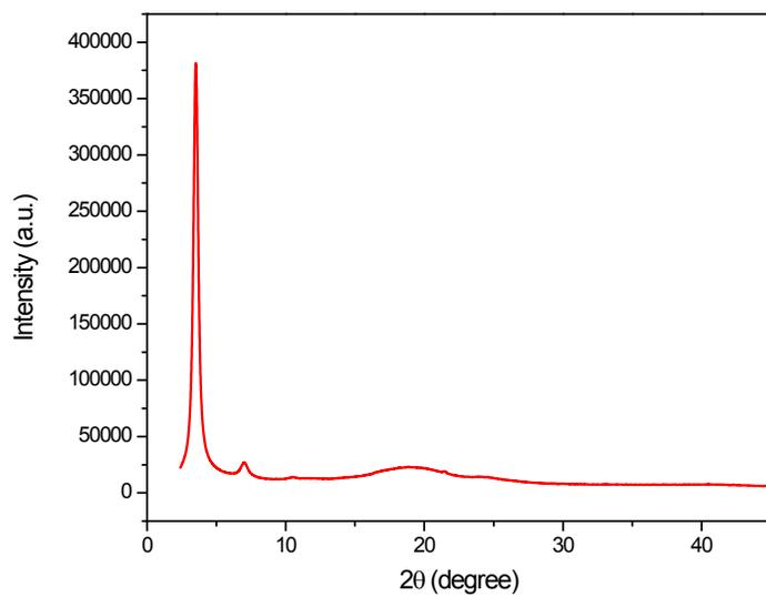
**Fig. S16** Transmission XRD pattern of **P2** flakes stacked between two Mylar substrates.
