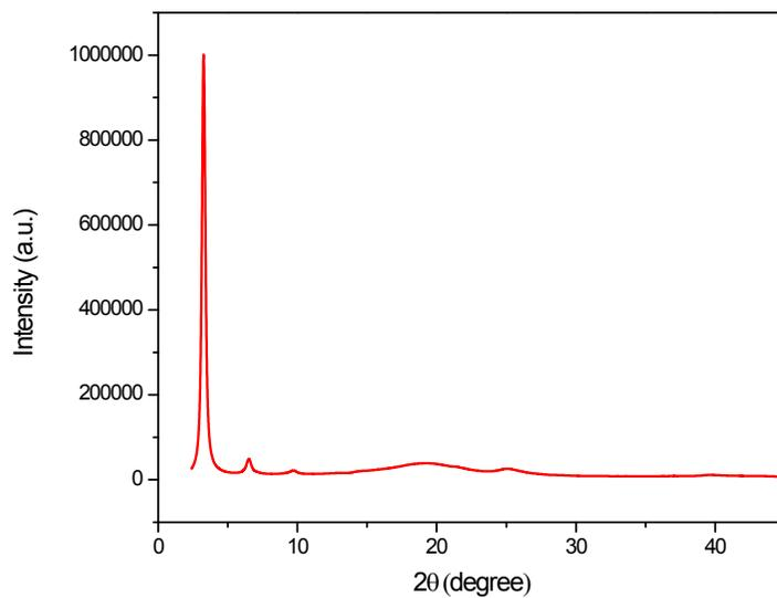
**Fig. S15** Transmission XRD pattern of **P1** flakes stacked between two Mylar substrates.
