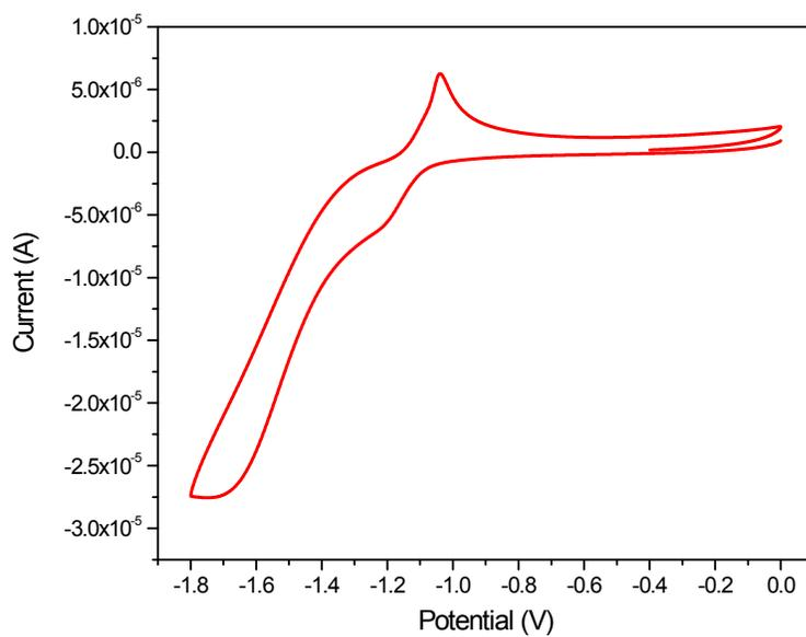
**Fig. S14** The reduction cyclic voltammogram of a **P1** thin film at a scan rate of  $0.100 \text{ V s}^{-1}$ .
