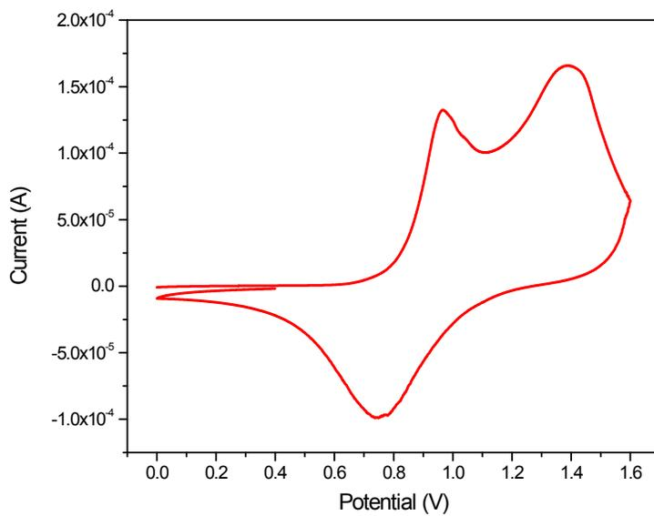
**Fig. S15** The oxidation cyclic voltammogram of a **P1** thin film at a scan rate of  $0.100 \text{ V s}^{-1}$ .
