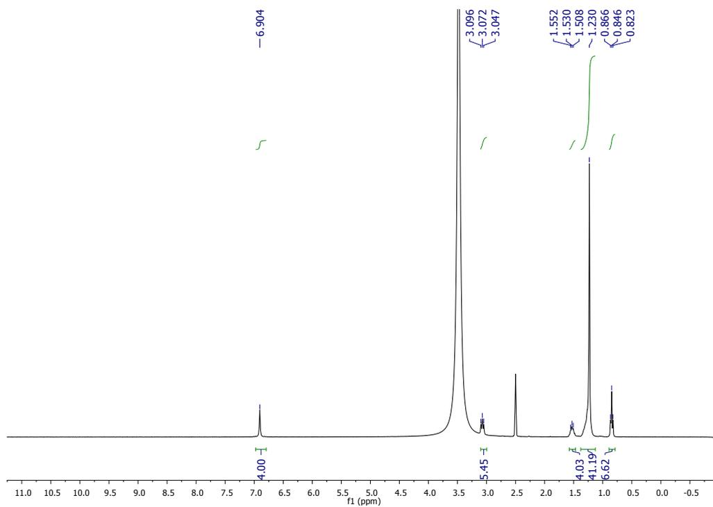
**Fig. S4** 300 MHz  $^1\text{H}$  NMR spectrum for *N,N'*-didodecylbenzene-1,4-diamine (**1**) in DMSO- $d_6$ .
