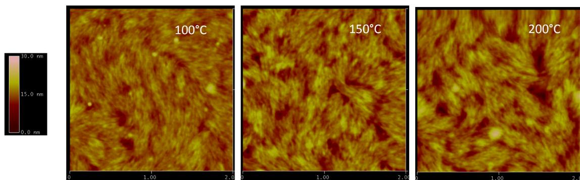
**Fig. S17** AFM images (2 μm × 2 μm each) of **P1** thin films on SiO<sub>2</sub>/Si substrates annealed at different temperatures.
