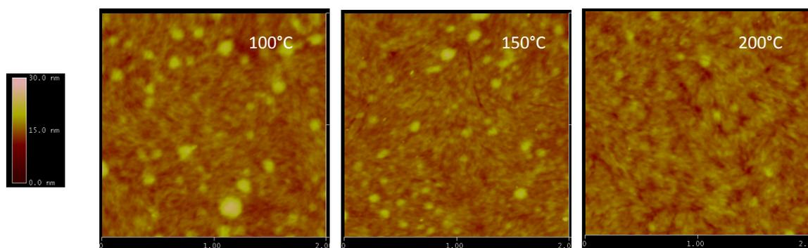
**Fig. S18** AFM images (2 μm × 2 μm each) of **P2** thin films on SiO<sub>2</sub>/Si substrates annealed at different temperatures.
