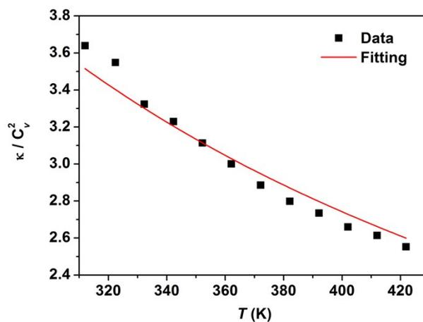
**Fig. S7** The plot of  $\kappa$  divided by  $C_v^2$  vs. temperature. The non-linear fitting using the function of  $y = ax^b$  give the constant  $A = 1096.82 \text{ g}^2 \text{ K}^2 \text{ J}^{-1} \text{ s}^{-1} \text{ m}^{-1}$ .
