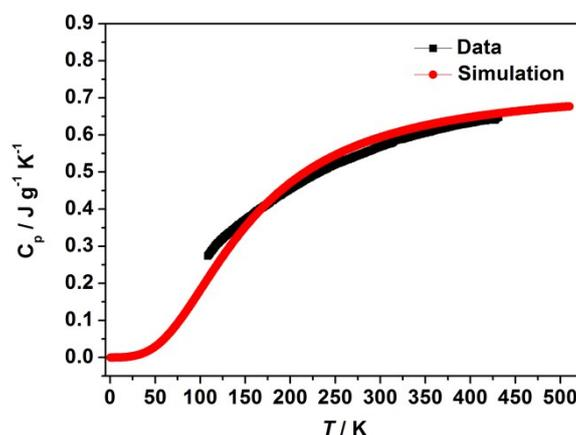
**Fig. S6** The calculated curve (Red) using  $T_D = 620$  K matches the measurement result perfectly.
