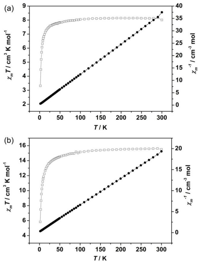
**Fig. S2** Plots of temperature dependence of  $\chi_M T$  ( $\square$ ) and  $\chi_M^{-1}$  ( $\bullet$ ) for **1** and **2** under 1000 Oe dc field between 2 and 300 K.
