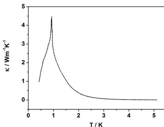
**Fig. S8** temperature-dependent thermal conductivity for compound **1** between 0.43-5.1K
