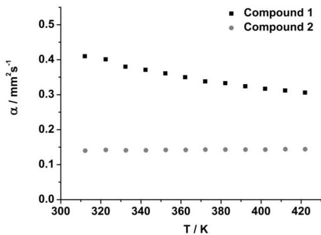
**Fig. S5** The thermal diffusion coefficient of compounds **1** and **2** between 312 and 352K.
