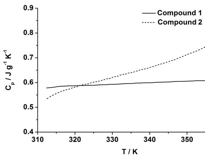
**Fig. S4** Specific heat capacity at indicated temperatures for compounds **1** and **2**.
