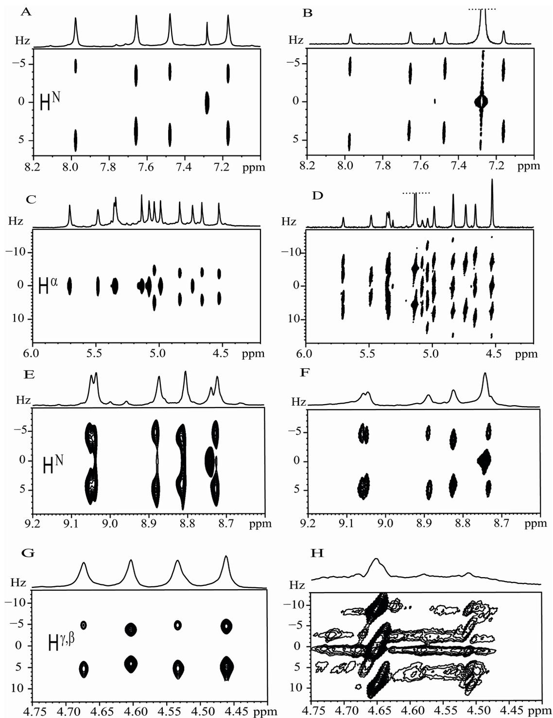
**Figure S1:** A, B, C, D cyclosporine A and E, F, G, H the heptapeptide. A, C, E, G the BSD SERF maps on  $H^N$ - $H^\alpha$ ,  $H^\alpha$ - $H^N$ ,  $H^N$ - $H^{\gamma/\beta}$ ,  $H^{\gamma/\beta}$ - $H^N$  respectively and B, D, F, H, the J-resolved after 45° tilting maps on  $H^N$ - $H^\alpha$ ,  $H^\alpha$ - $H^N$ ,  $H^N$ - $H^{\gamma/\beta}$ ,  $H^{\gamma/\beta}$ - $H^N$  respectively.
