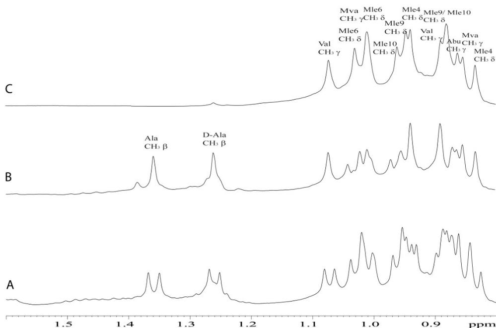
**Figure S3:** A) standard  $^1\text{H}$  1D spectrum, Band selective homodecoupling 1D by replacing the SERF block by its first EBURP  $90^\circ$  pulse (see Figure 1 of the main text) B) using 10 ms (400 Hz) EBURP / REBURP pulses, and C) using 20 ms (200 Hz) EBURP / REBURP pulses.
