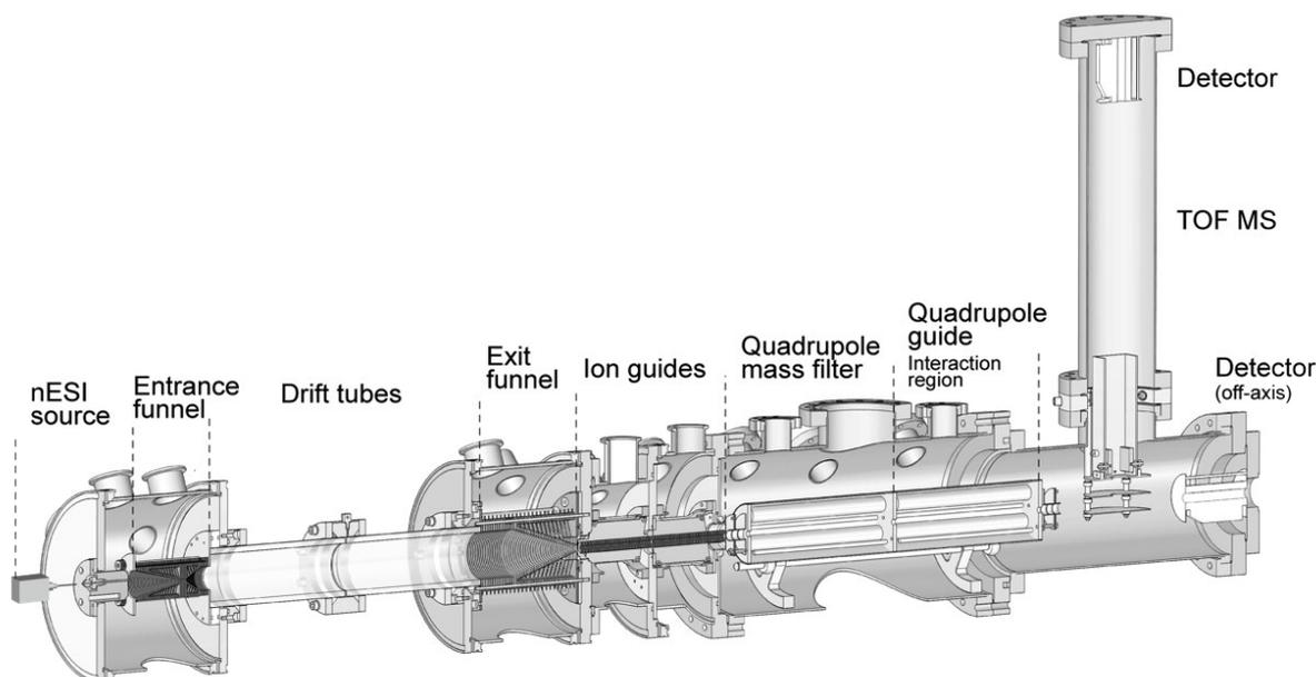
**Fig.ES4:** Instrumental setup of the DT instrument.<sup>5</sup>
