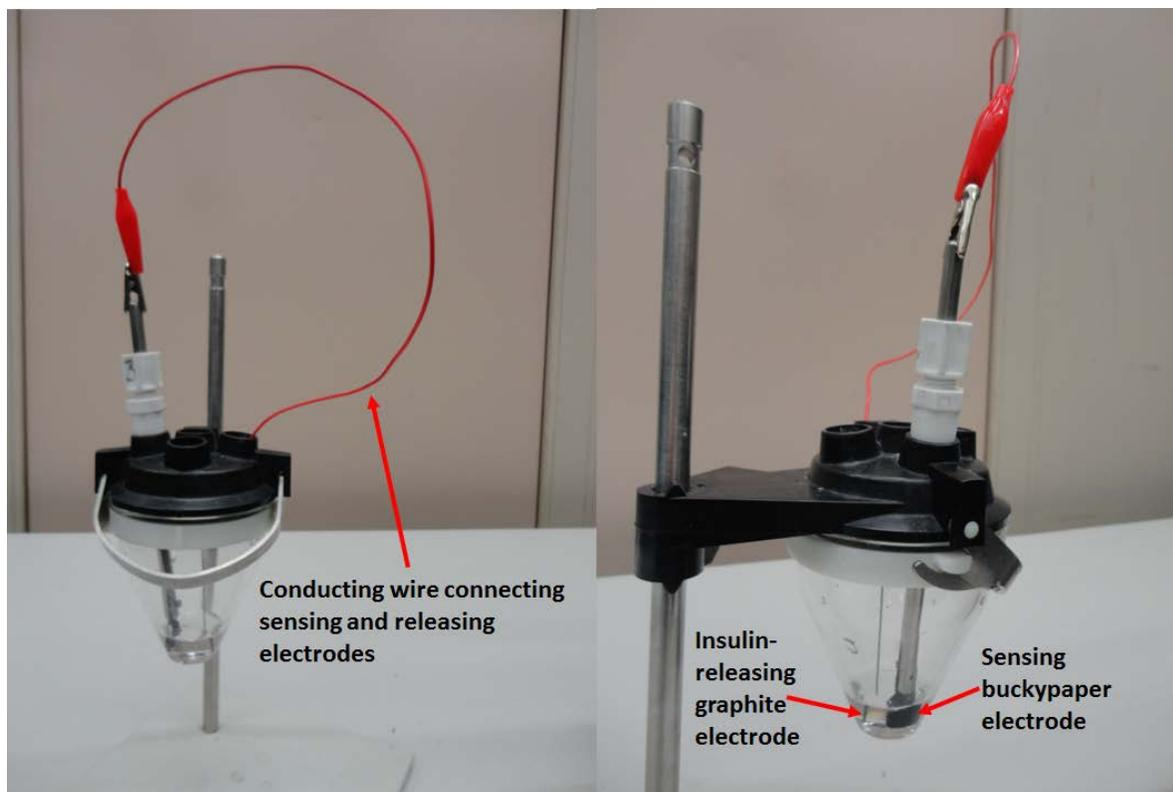
**Figure S4.** Experimental setup. Electrically connected sensing and releasing electrodes in the cell.
