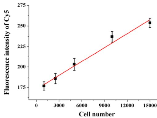
**Fig. S2** The linear correlation between Cy5 fluorescence intensity and the cell number in the range from 1000 to 15000. Error bars show the standard deviation of three experiments.
