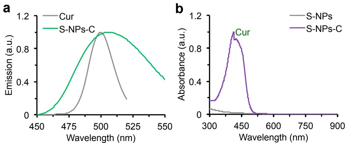
**Fig. S2** Encapsulation of curcumin (Cur or C) in S-NPs-C using single-emulsion method. (a) Fluorescence spectra of emission (excitation: 420 nm) of free Cur and S-NPs-C. (b) UV-Vis absorbance of S-NPs and S-NPs-C (in DI water). The data show successful encapsulation of Cur in the S-NPs-C produced using the single-emulsion method.
