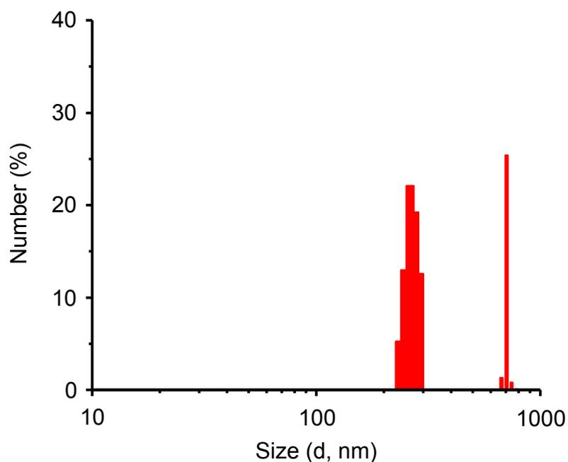
**Fig. S1** Size distribution of NPs made of PLGA alone using the double-emulsion method in DI water determined by dynamic light scattering (DLS): two peaks show up because the PLGA NPs of 262 nm tend to form aggregates of 707 nm, probably due to the hydrophobic nature of their surface that drives the smaller PLGA nanoparticles to stick together in the hydrophilic environment of DI water to minimize interfacial energy.
