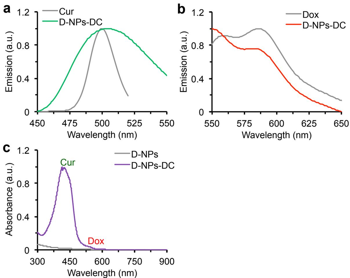
**Fig. S3** Encapsulation of doxorubicin (Dox, or D) and curcumin (Cur or C) in D-NPs-DC using double-emulsion method. Fluorescence spectra of emission from (a) free Cur and D-NPs-DC (excitation: 420 nm) and (b) Dox and D-NPs-DC (excitation: 486 nm). (c) UV-Vis absorbance of D-NPs without encapsulating any agents and D-NPs-DC (in DI water). The data show successful encapsulation of Cur and Dox in the D-NPs-DC produced using the double-emulsion method.
