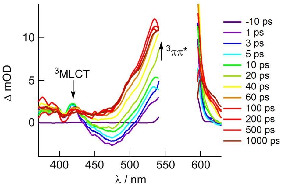
**Figure S5.** Ultrafast transient absorption spectra of **2** in  $\text{CH}_3\text{CN}$  with  $\lambda_{\text{exc}} = 568 \text{ nm}$  (fwhm = 300 fs).
