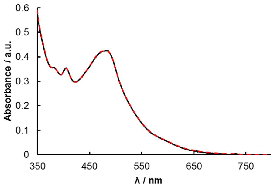
**Figure S3.** Electronic absorption spectrum of **1** in  $\text{CH}_3\text{CN}$  in the dark initially (black) and after 24 hours (red).
