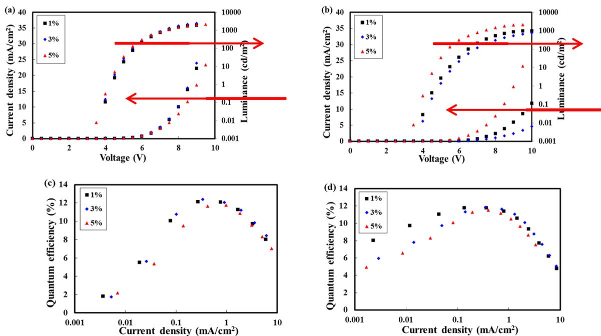
140 Figure S6. Current density–voltage–luminance curves of (a) BFCz-2CN and (b) BTCz-2CN at different doping concentrations. Quantum efficiency–current density curves of (c) BFCz-2CN and (d) BTCz-2CN at different concentrations.
