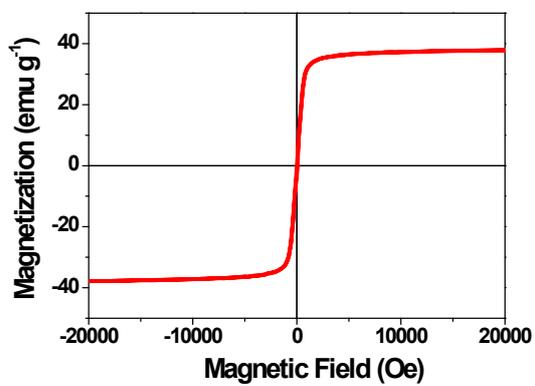
**Figure S2.** Mass magnetization curve of the  $\text{Fe}_3\text{O}_4$  nanoparticles. The particles were superparamagnetic at room temperature with no remnant magnetization.
