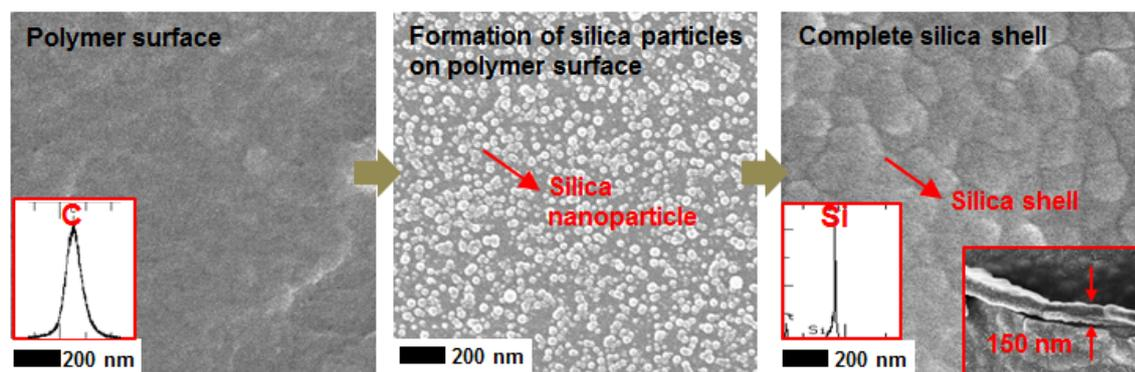
**Figure S4.** FE-SEM images showing silica shell growth on a copolymer microparticle with different silica coverage. Initially, the seed silica nanoparticles increase in size as the reaction proceeds. Eventually, the seed nanoparticles coalesce and form a continuous silica shell on the copolymer surface. The inset shows the thickness of the silica layer, which was approximately 150 nm.
