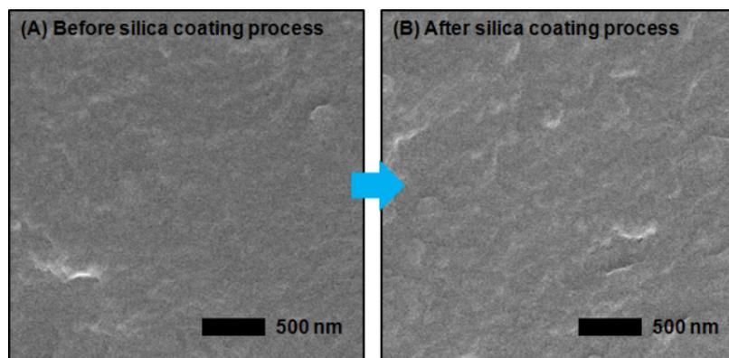
**Figure S3.** FE-SEM images of polymeric microparticles before (A) and after (B) the silica-coating process. The polymeric microparticles were generated without silane-grafting materials. Therefore, a silica layer was not formed on the surface of the polymeric microparticles after the silica coating process.
