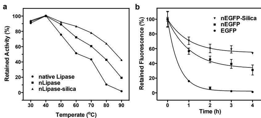
Fig. S5 (a) Relative activity of native lipase, nLipase and nLipase-silica at different temperature; b) relative activity of native EGFP, nEGFP and nEGFP-silica at 75 °C.
