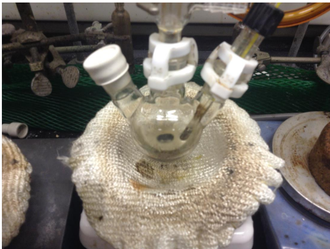
S.I. Figure 5. Reaction vessel after reaction of \text{Ga}(\text{acac})_3 and 2 molar equivalents of Oleylamine at 320 °C for 1 hour. White powder next to stir bar is unreacted \text{Ga}(\text{acac})_3 and no visible color change occurs, indicating no reaction.
