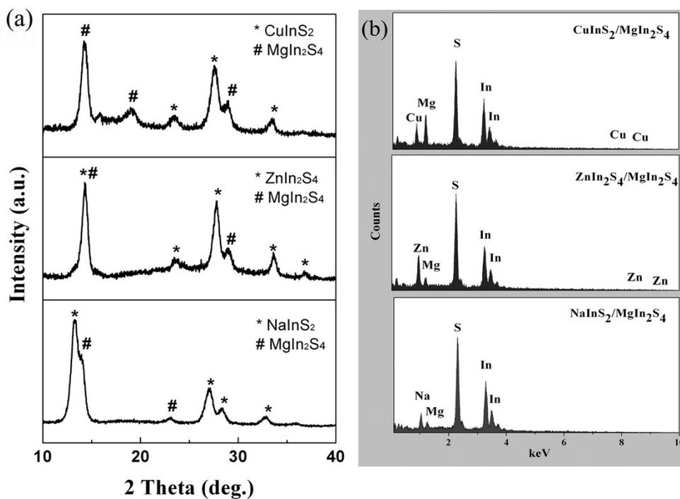
**Figure S6** (a) XRD and (b) EDX spectra of other ternary sulfide heterogeneous structures CuInS<sub>2</sub>/MgIn<sub>2</sub>S<sub>4</sub>, ZnIn<sub>2</sub>S<sub>4</sub>/MgIn<sub>2</sub>S<sub>4</sub> and NaInS<sub>2</sub>/MgIn<sub>2</sub>S<sub>4</sub>.
