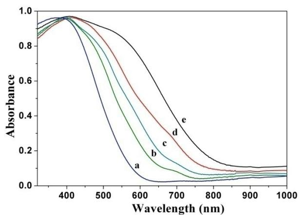
**Figure S7** UV-vis spectra of heterogeneous nanosheets with different molar ratio of Cu/Na by ion exchange reaction: (a) 0 %, (b) 0.3 %, (c) 0.5 %, (d) 1 % and (e) 1.5%.
