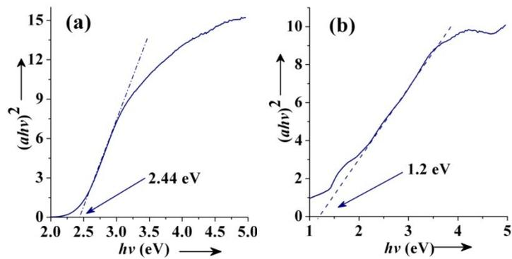
**Figure S8** (a) bandgap energy of the pure  $\text{NaInS}_2$  and b)  $\text{CuInS}_2$ .
