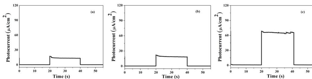
**Figure S10** Photocurrent-time plots for the working electrodes of (a) pure  $\text{NaInS}_2$ , (b)  $\text{CuInS}_2$  nanoparticles decorated  $\text{NaInS}_2$  and (c)  $\text{CuInS}_2/\text{NaInS}_2$  integrated heterostructures, with a bias of 0.2 V in 0.1 M  $\text{K}_2\text{SO}_4$  chopped AM1.5 illumination, 100  $\text{mW}/\text{cm}^2$ .
