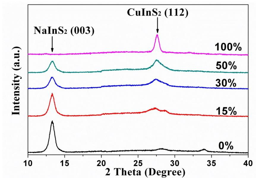
**Figure S3** XRD patterns of heterogeneous nanosheets with different molar ratio of Cu/Na by an ion exchange reaction.
