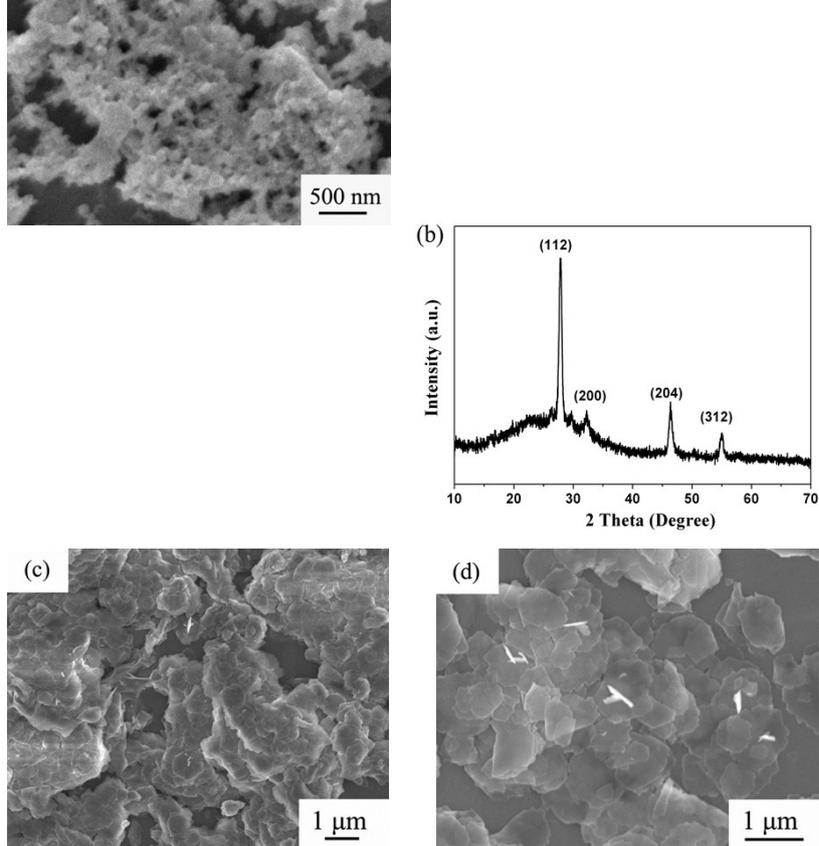
**Figure S9** (a) SEM image and (b) XRD pattern of synthesized  $\text{CuInS}_2$  nanoparticles, (c) and (d) SEM images of obtained  $\text{CuInS}_2$  nanoparticles (0.5%) decorated  $\text{NaInS}_2$  heterogenous photocatalysts.
