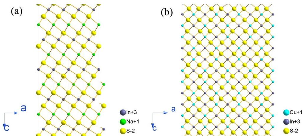
**Figure S5** The schematic illustration of the atom arrangement of (a) NaInS<sub>2</sub> and (b) CuInS<sub>2</sub>, with (010) plane.
