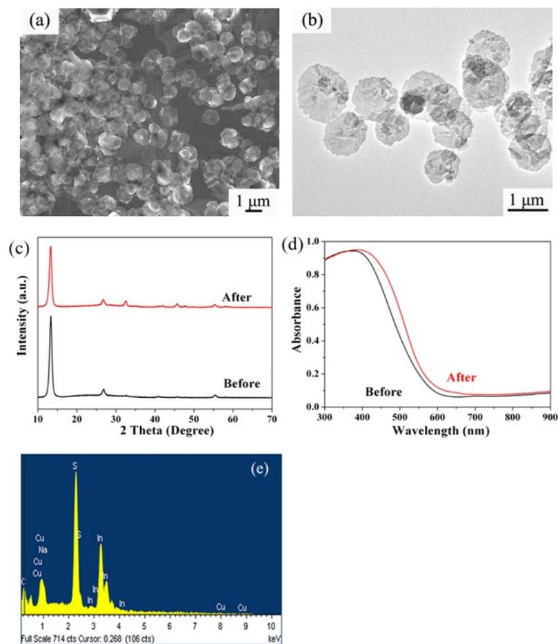
**Figure S2** (a) SEM and (b) TEM images, (c) XRD, (d) UV-vis and (e) EDX pattern of obtained nanosheets reacted with 5 %  $\text{Cu}^+$  ions at room temperature.
