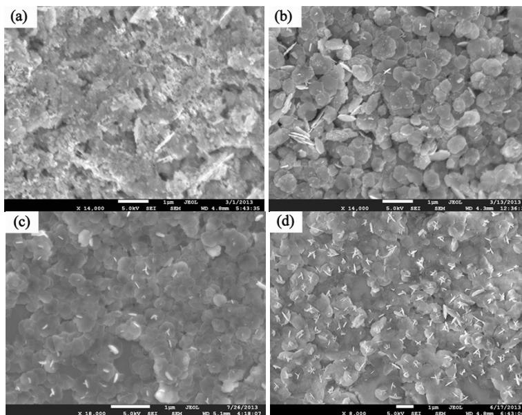
**Figure S1** Typical morphological evolution of NaInS<sub>2</sub> nanoparticles with different reaction times: (a) 20 min., (b) 1 h, (c) 5 h and (d) 12h.
