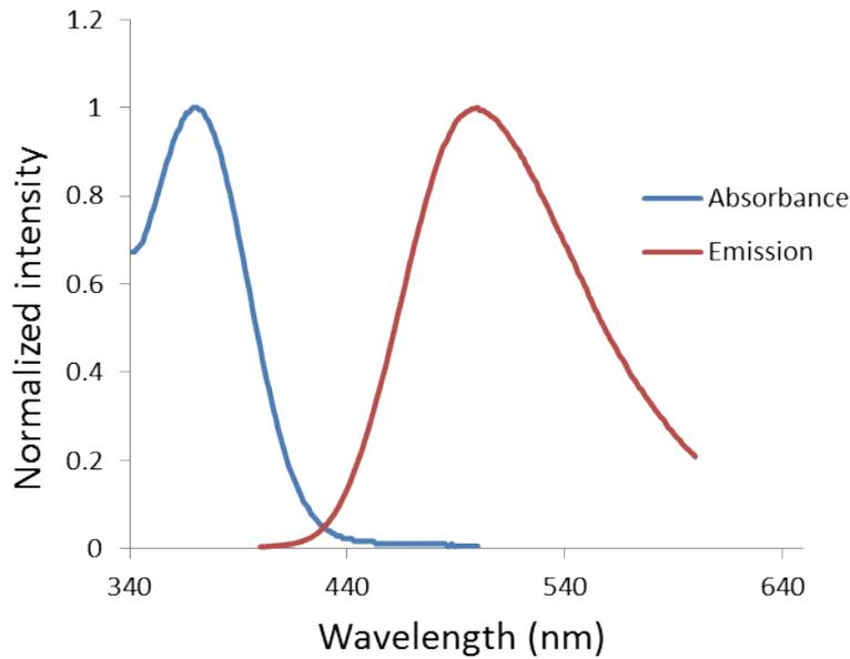
**Fig. S1** Normalized absorbance and emission profiles of **CDb12** in DMSO.
