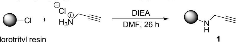
DIEA (6.45 g, 50 mmol) was added to a solution of propargylamine hydrochloride (910 mg, 10 mmol) in DMF. Then the chlorotriyl resin (1 g, 1.37 mmol/g) was added to this solution and was shaken for 26 hours. The resin was washed then with DMF, MeOH and DCM (5 times each). After washing the resin was quenched with 40% MeOH in DMF for 1 hour. Finally, the resin was washed with DMF, MeOH and DCM (5 times each) and dried under high vacuum.
