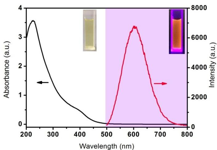
Figure S2. UV-Vis adsorption (black) and fluorescence spectrum (red) of Au NCs solution. The excitation wavelength is 365 nm. Insets are Au NCs solution under white light (left) and UV light (right) irradiation.
