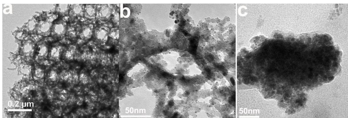
Figure S4. TEM images of Au NCs/TiO<sub>2</sub> photonic array (a and b) and Au NCs (c) after catalysis reaction. The comparison results indicate that aggregation of Au NCs is suppressed by loading on TiO<sub>2</sub> photonic array.
