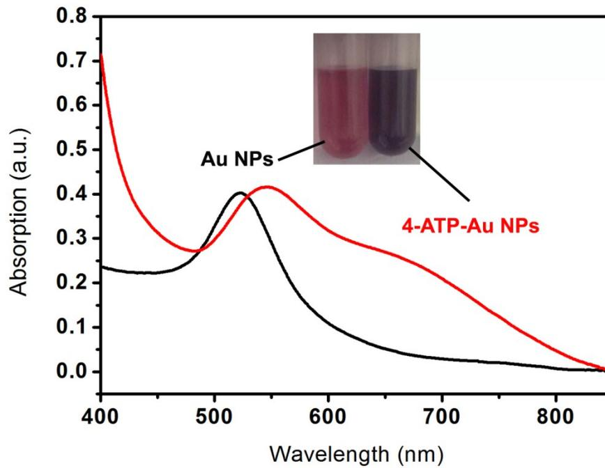
Figure S8. Absorption spectra of colloidal Au NPs (20 nm) mixed with ethanol (black curve) and 4-ATP ethanol solution (red curve).
