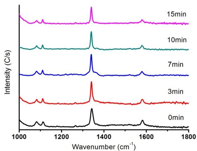
Figure S3. Raman spectra for monitoring the reduction of 4-NTP on TiO<sub>2</sub> photonic array without Au NCs.
