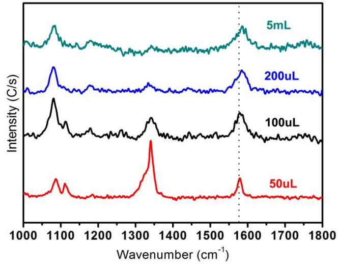
Figure S7. Raman spectra of 4-NTP reduced by different amount of  $\text{NaBH}_4$  solution after 7 min on Au NCs/ $\text{TiO}_2$  photonic array.
