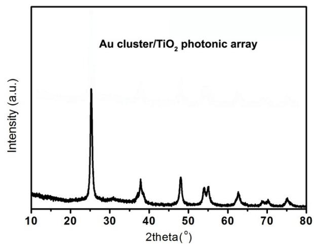
Figure S5. XRD pattern of Au NCs/TiO<sub>2</sub> photonic microarray. The patterns are attributed to anatase, and Au signals are not observed because of its tiny crystallite size.
