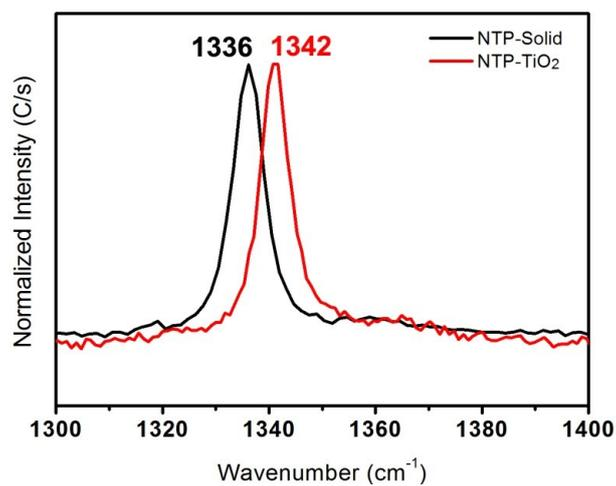
Figure. S6 Raman spectra of 4-NTP solid and 4-NTP adsorbed on TiO<sub>2</sub>
