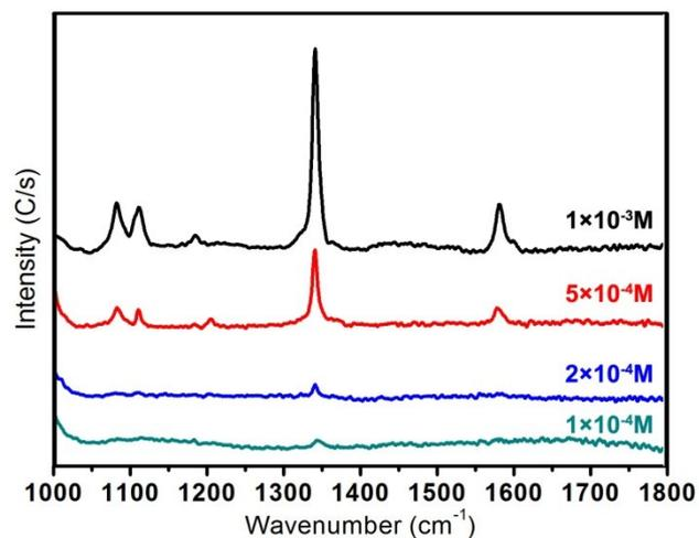
Figure S1. Raman spectra of 4-NTP with different concentrations adsorbed on  $\text{TiO}_2$  photonic array.
