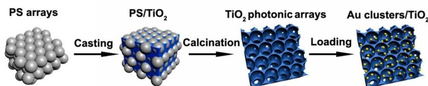
Scheme 1. Synthesis process of Au NCs/TiO<sub>2</sub> photonic array.
